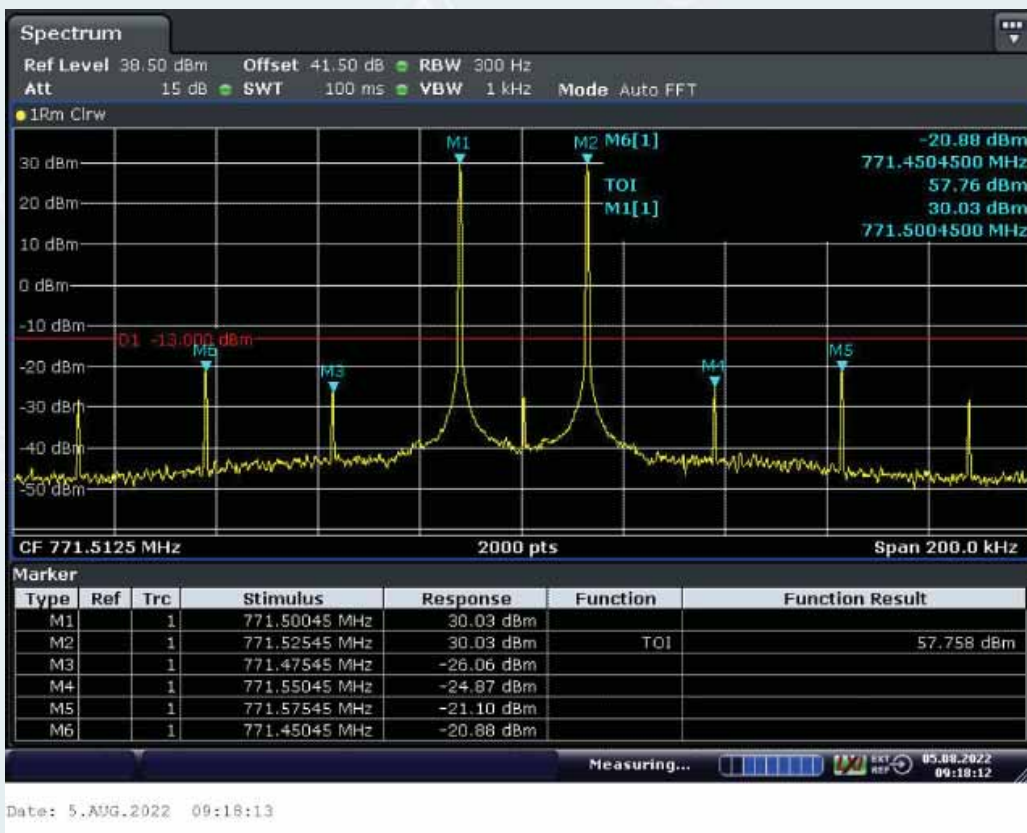
Mid Frequency and with the input signal amplitude set 3 dB above the ALC threshold
