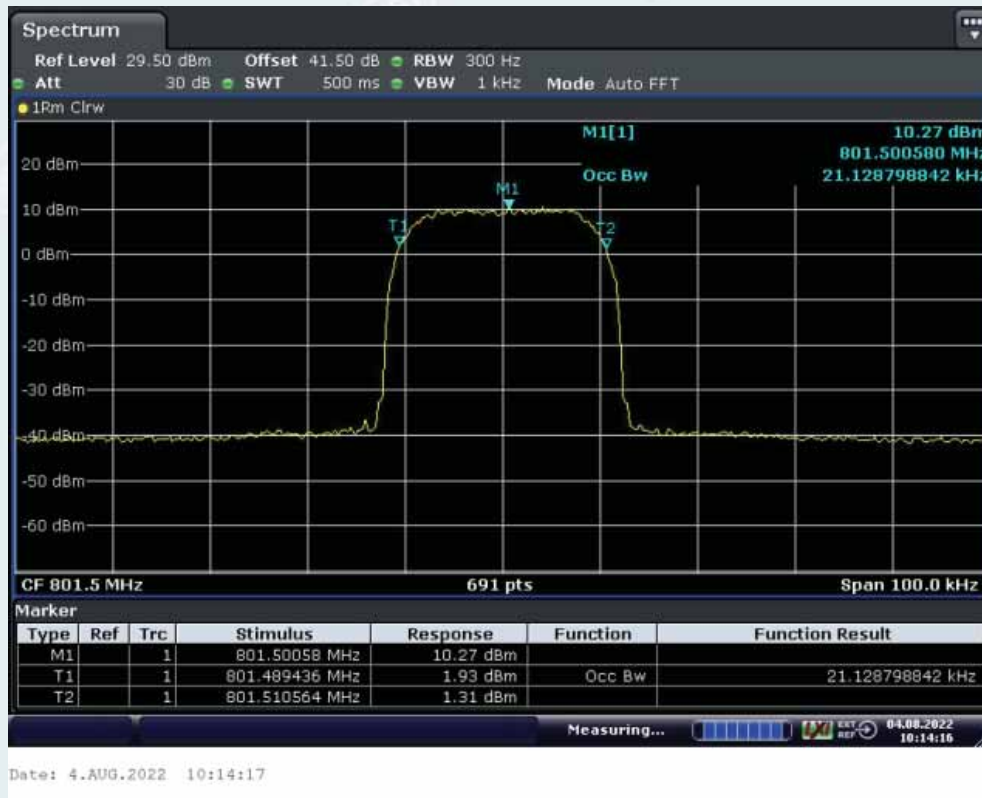
Middle Frequency: 801.5MHz, Output occupied BW(AGC)
