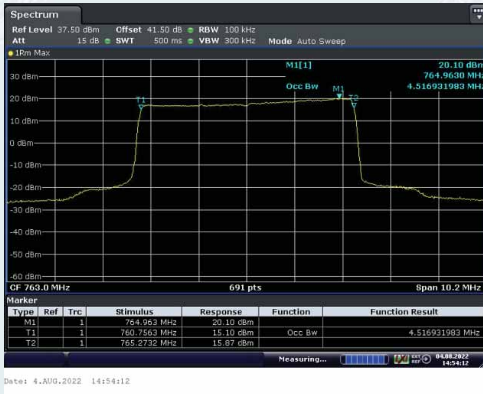
Middle Frequency: 763.0MHz, Output occupied BW(AGC)
