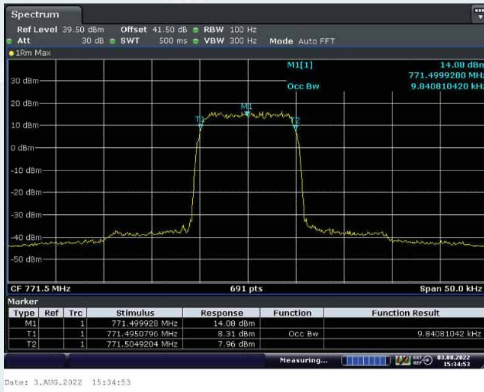
Middle Frequency: 771.5MHz, Output occupied BW (with the input signal amplitude set 3 dB above the AGC threshold)
