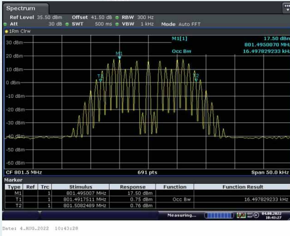
Middle Frequency: 801.5MHz, Output occupied BW(AGC)
