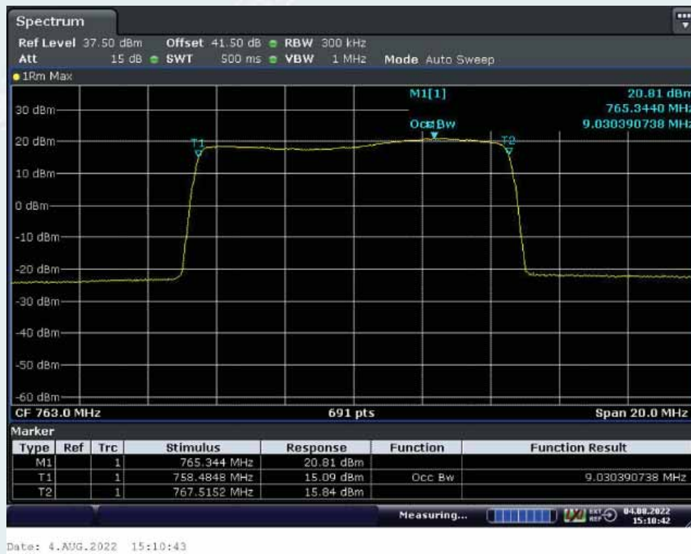
Middle Frequency: 763.0MHz, Output occupied BW (with the input signal amplitude set 3 dB above the AGC threshold)
