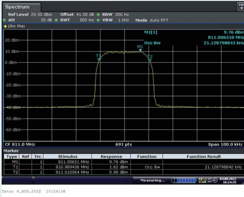
Middle Frequency: 811.0MHz, Output occupied BW(AGC)
