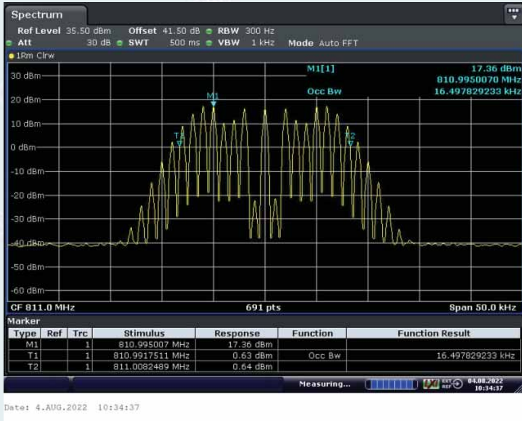
Middle Frequency: 811.0MHz, Output occupied BW(AGC)
