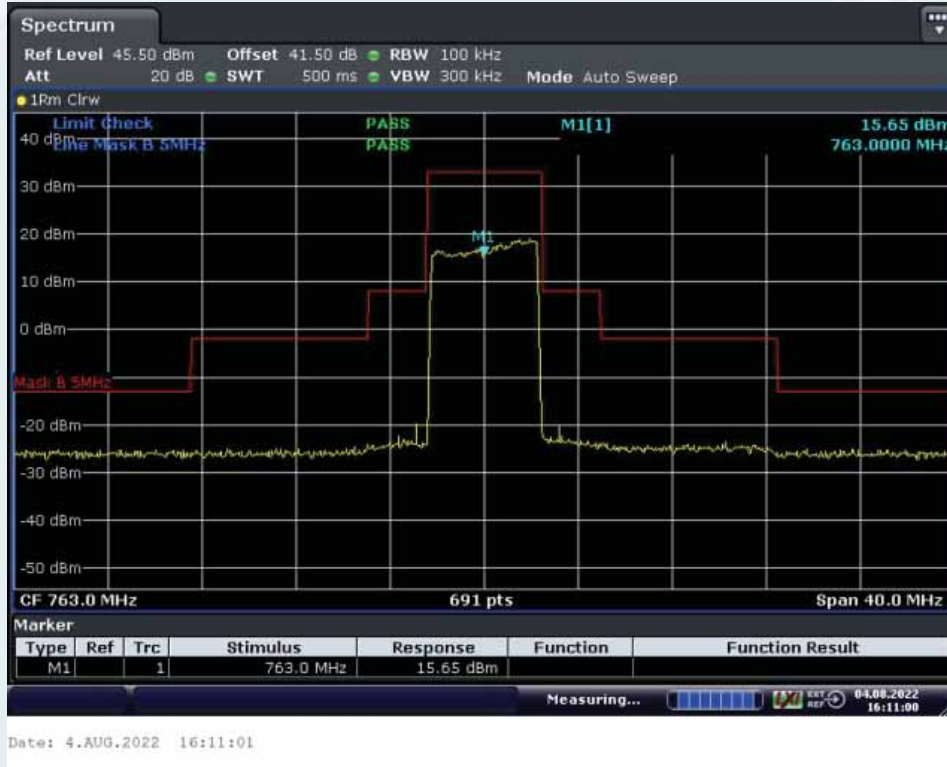
With the input signal amplitude set the AGC threshold Middle Frequency: 763.0MHz
