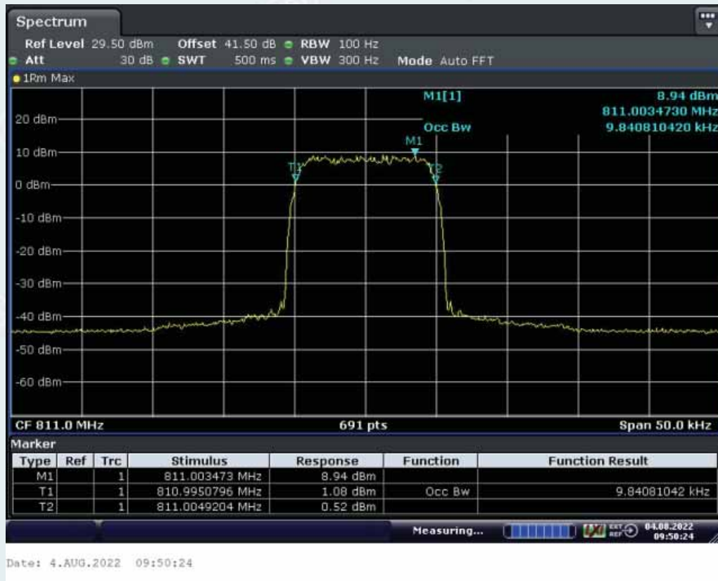
Middle Frequency: 811.0MHz, Output occupied BW(AGC)
