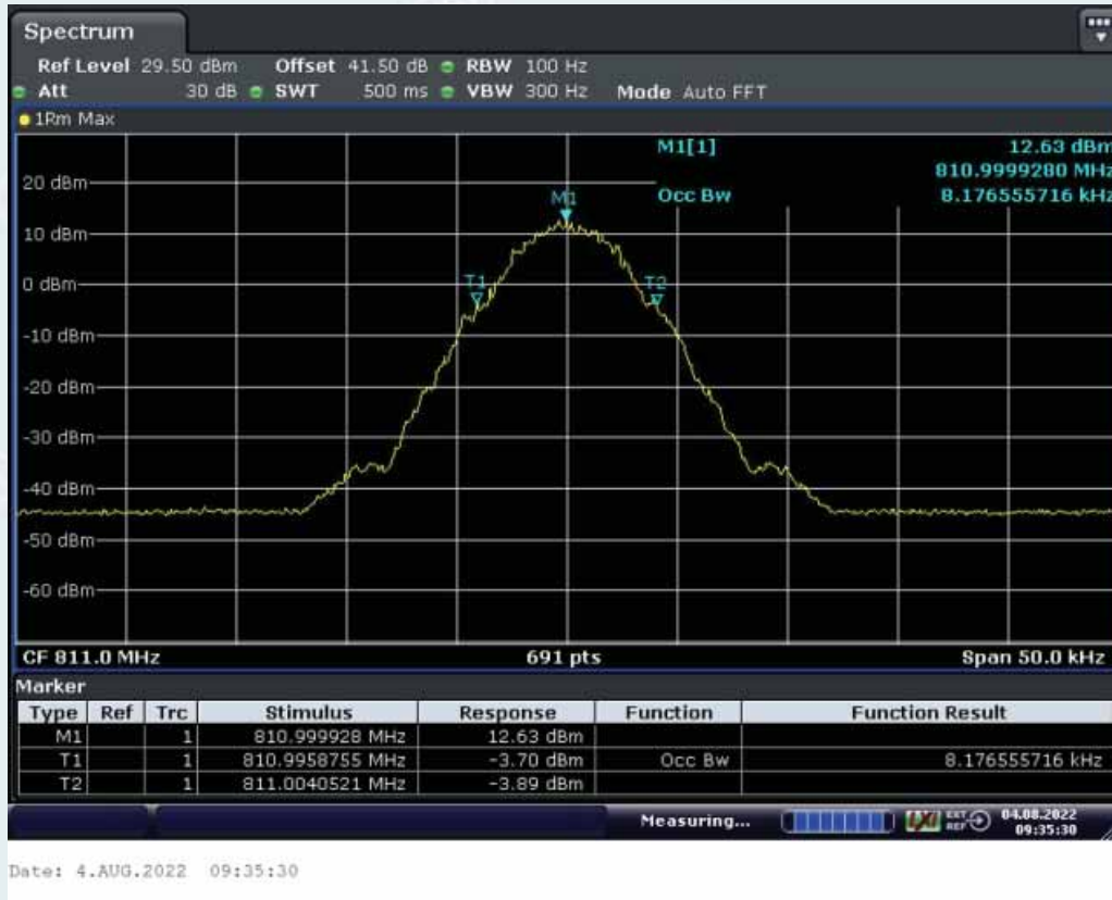
Middle Frequency: 811.0MHz, Output occupied BW(AGC)
