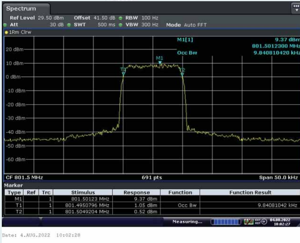
Middle Frequency: 801.5MHz, Output occupied BW(AGC)
