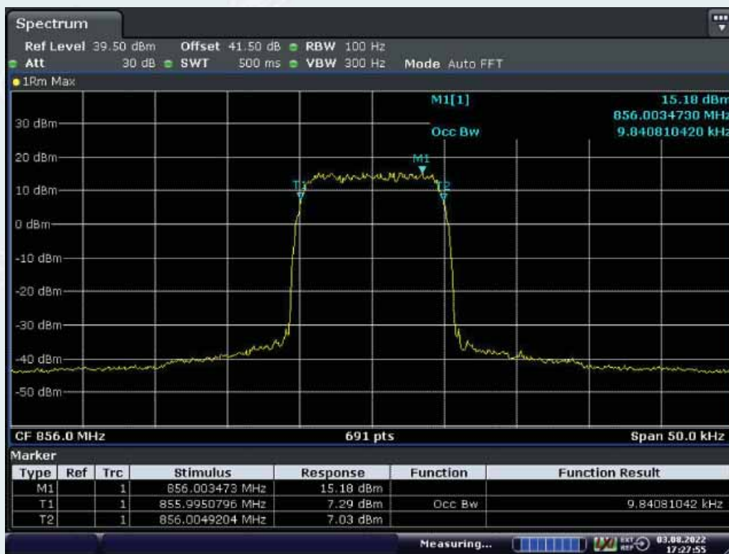
Middle Frequency: 856.0MHz, Output occupied BW (with the input signal amplitude set 3 dB above the AGC threshold)
