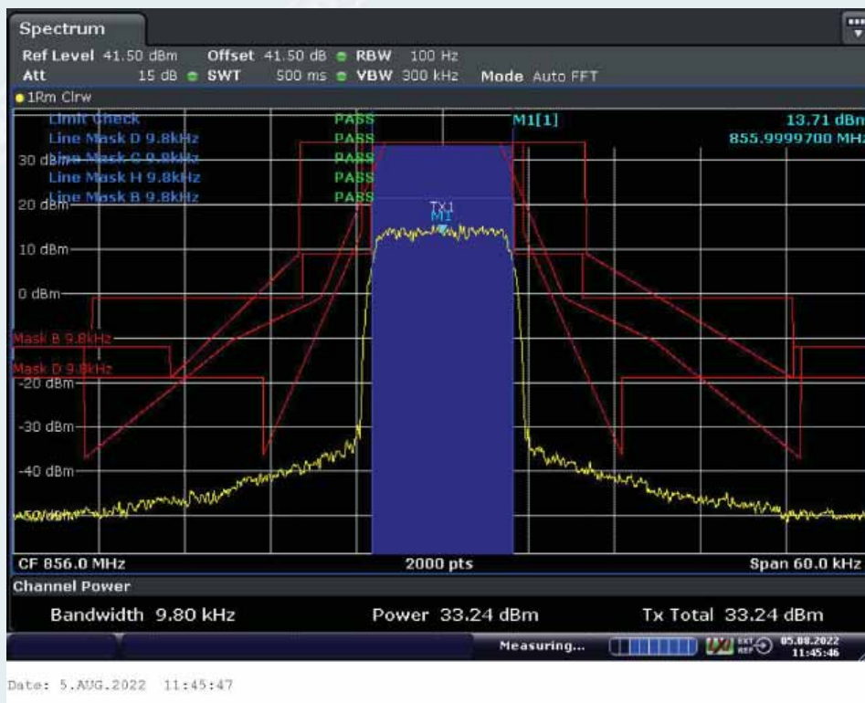
With the input signal amplitude set 3 dB above the AGC threshold Middle Frequency: 856.0MHz
