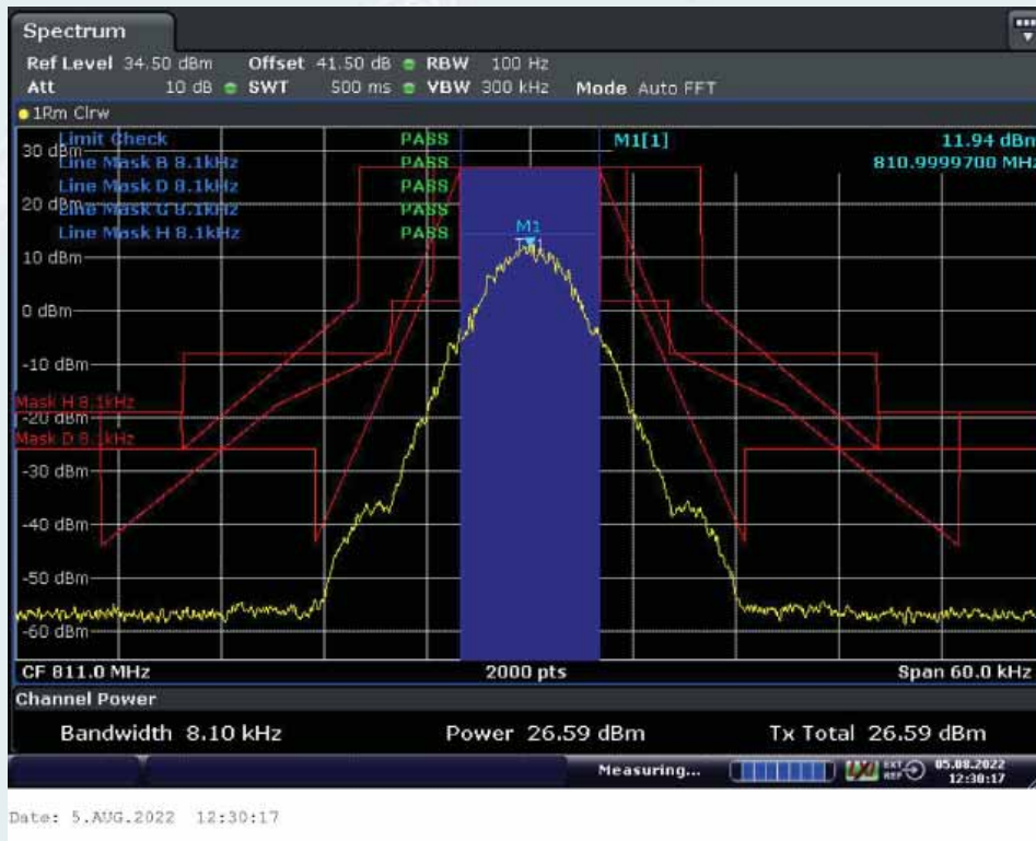
With the input signal amplitude set the AGC threshold Middle Frequency: 811.0MHz
