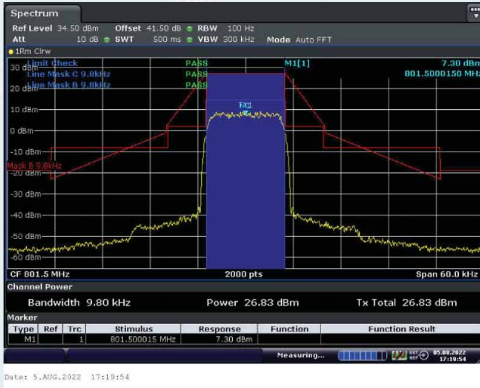
With the input signal amplitude set the AGC threshold Middle Frequency: 801.5MHz
