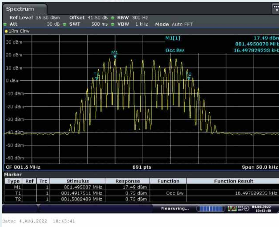
Middle Frequency: 801.5MHz, Output occupied BW (with the input signal amplitude set 3 dB above the AGC threshold)
