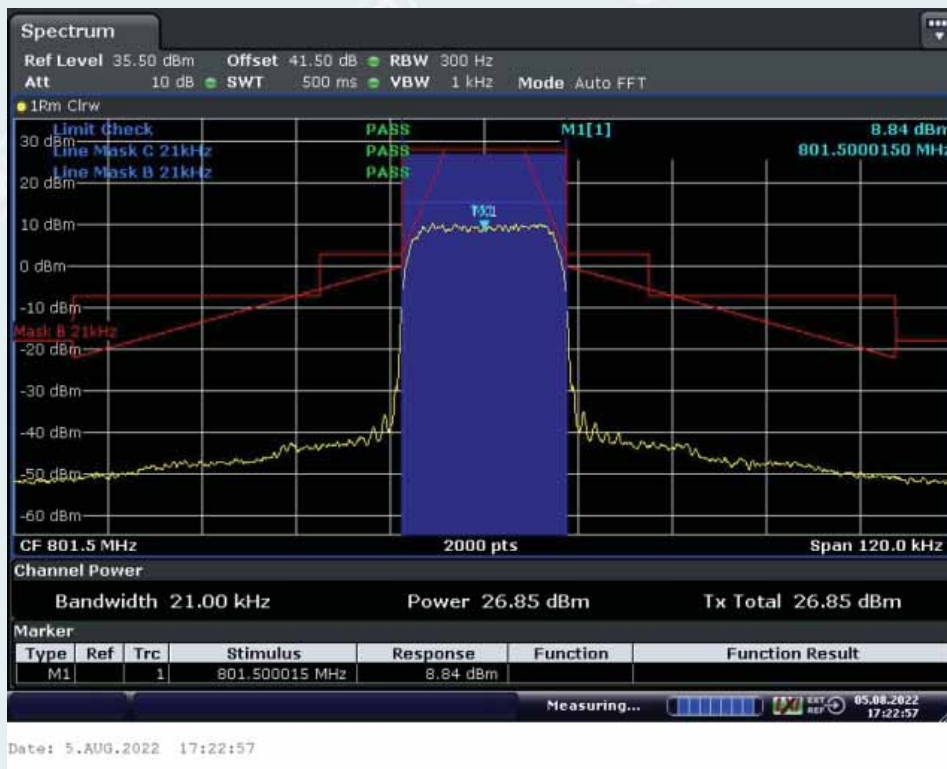
With the input signal amplitude set 3 dB above the AGC threshold Middle Frequency: 801.5MHz
