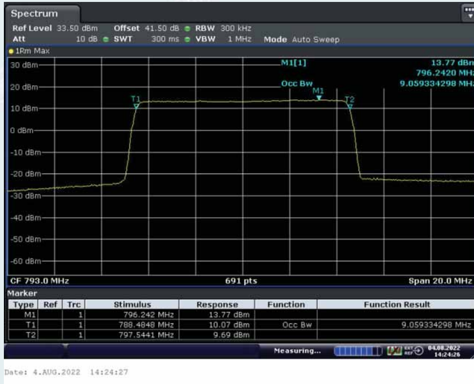
Middle Frequency: 793.0MHz, Output occupied BW(AGC)
