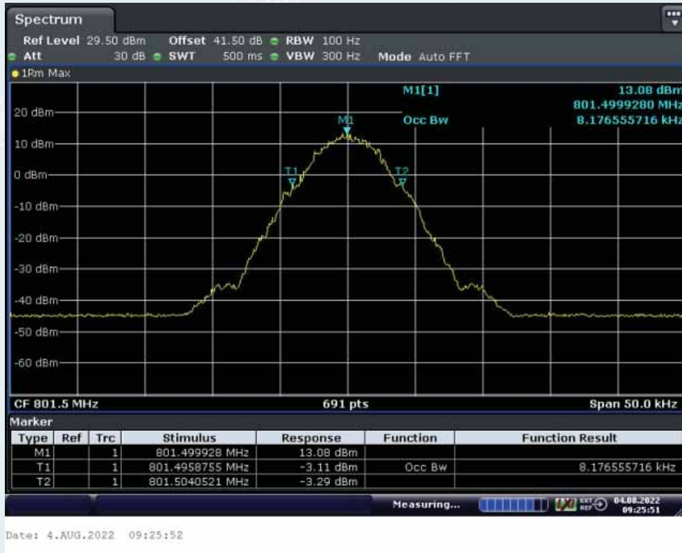
Middle Frequency: 801.5MHz, Output occupied BW(AGC)
