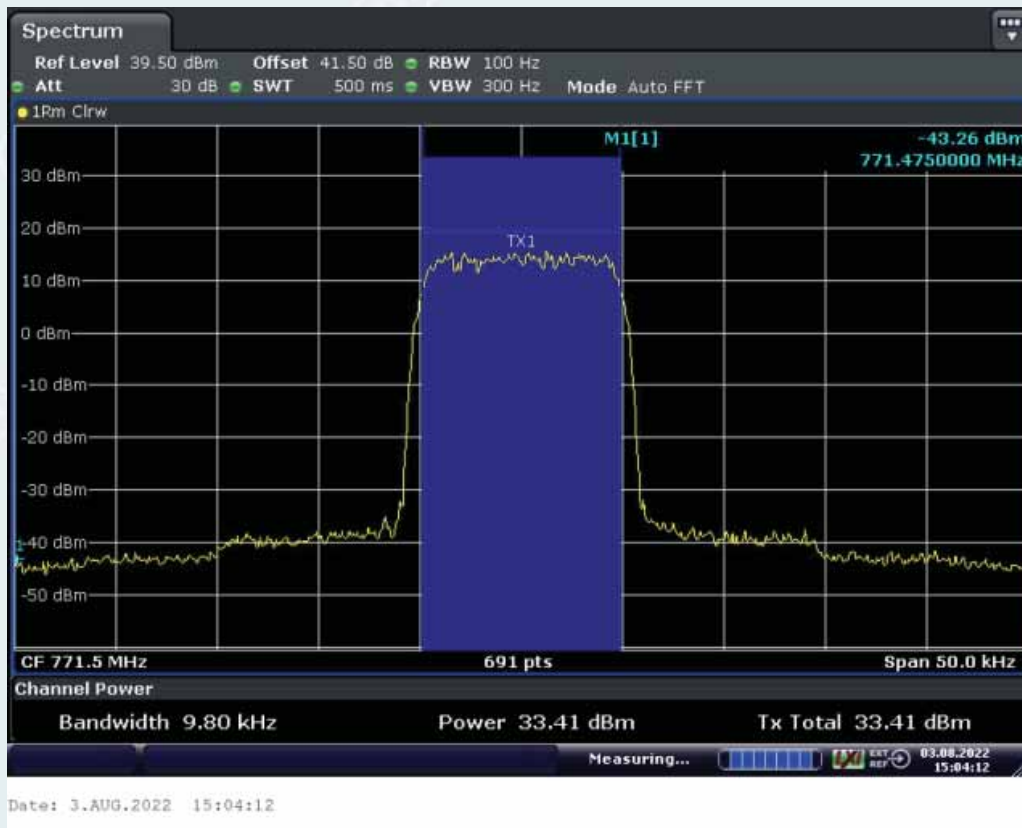
Middle Frequency: 771.5MHz, Output occupied BW(AGC)
