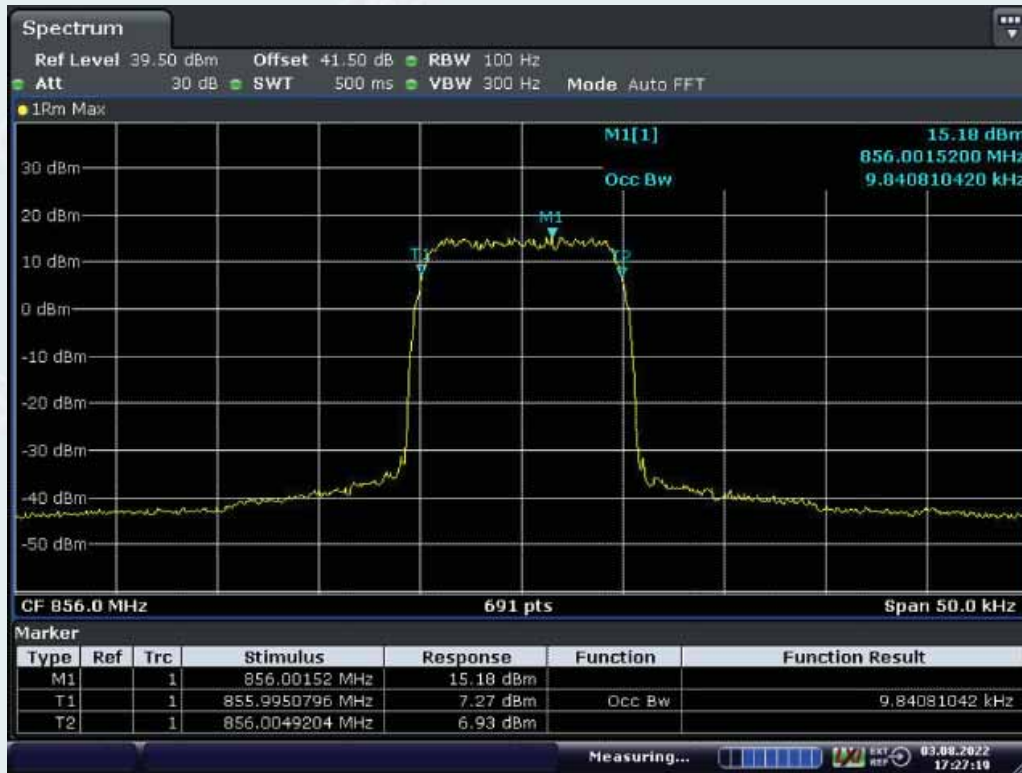
Middle Frequency: 856.0MHz, Output occupied BW(AGC)
