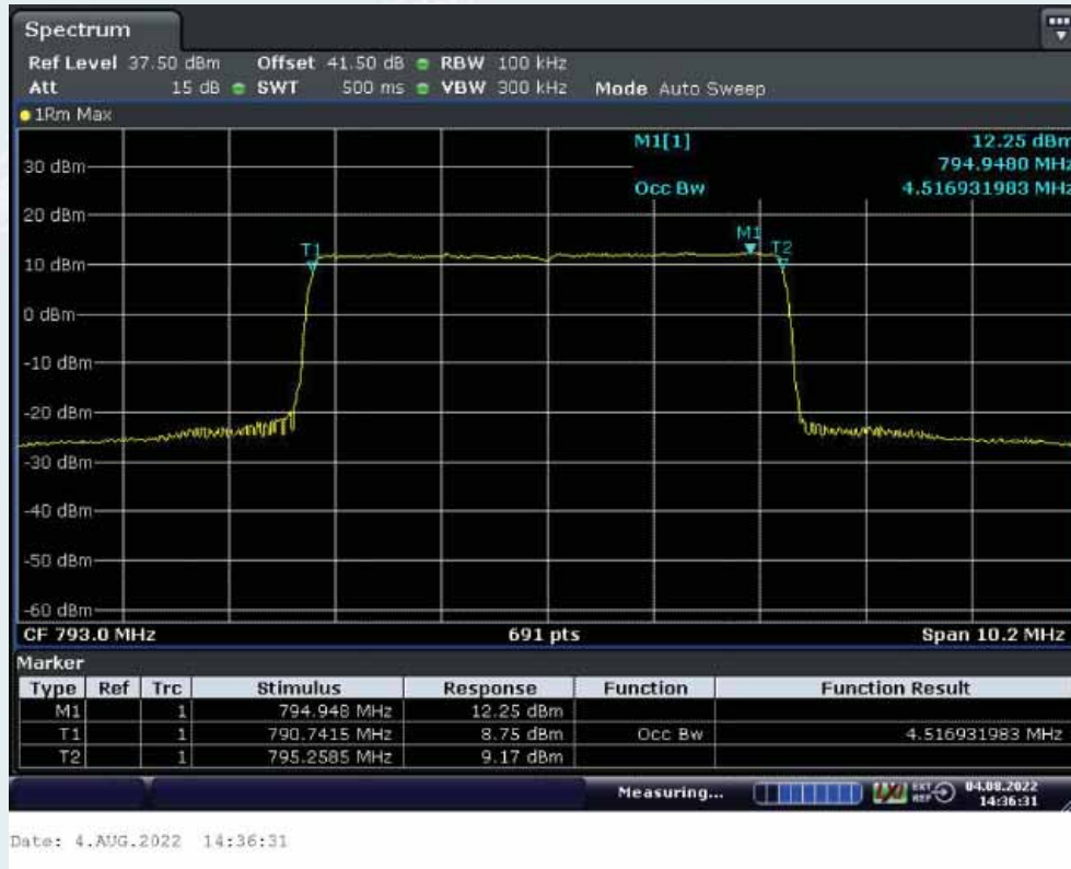
Middle Frequency: 793.0MHz, Output occupied BW(AGC)
