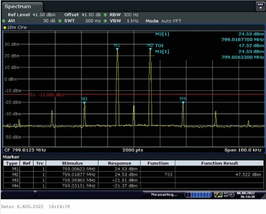
Low Frequency and with the input signal amplitude set 3 dB above the ALC threshold
