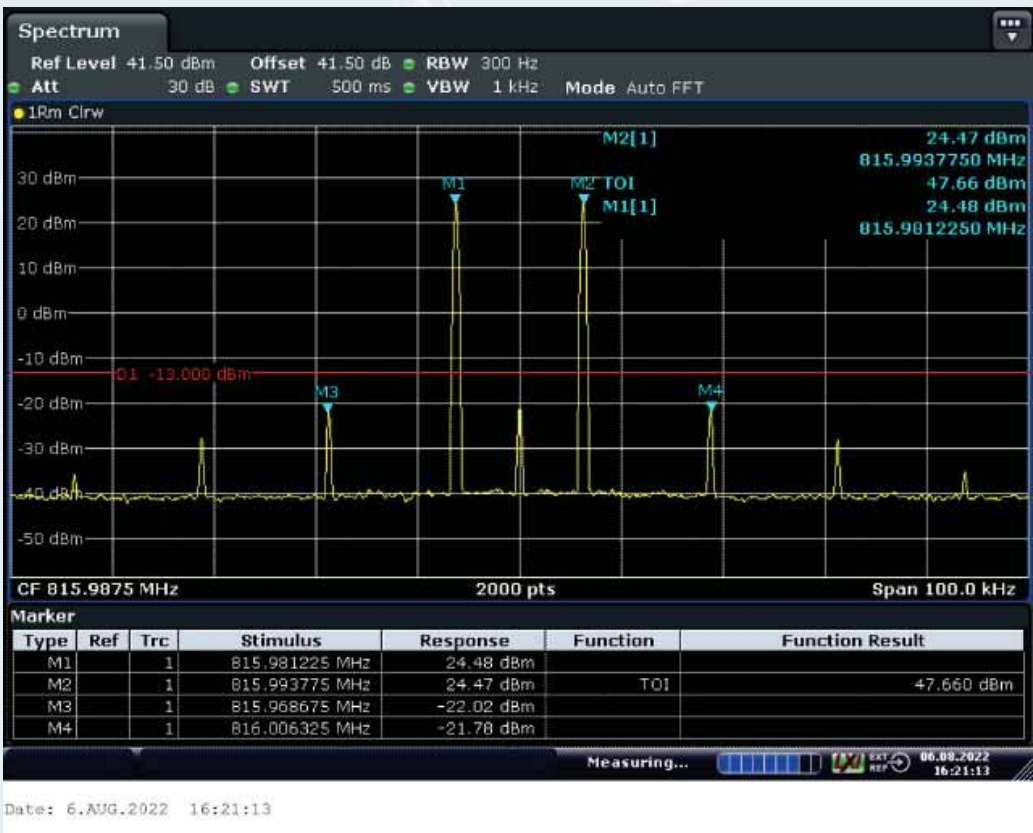
High Frequency and with the input signal amplitude set 3 dB above the ALC threshold
