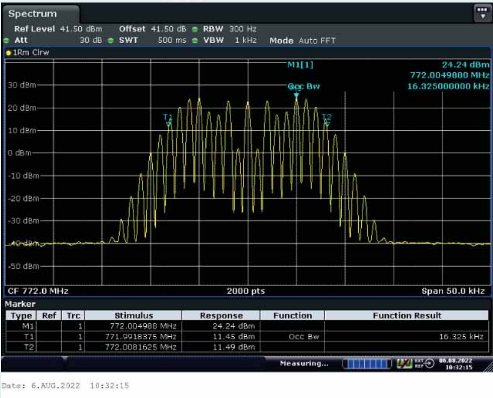
Middle Frequency: 772.0MHz, Output occupied BW (with the input signal amplitude set 3 dB above the AGC threshold)
