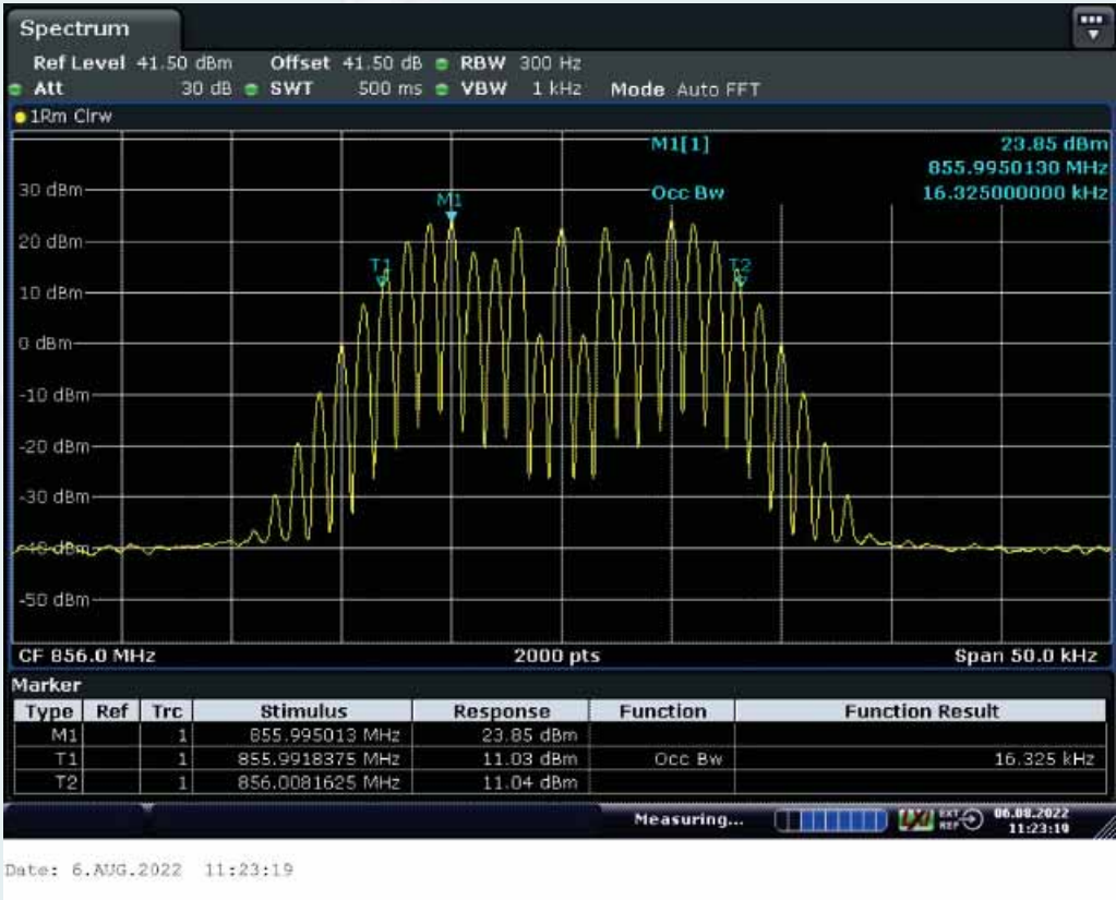
Middle Frequency: 856.0MHz, Output occupied BW (with the input signal amplitude set 3 dB above the AGC threshold)
