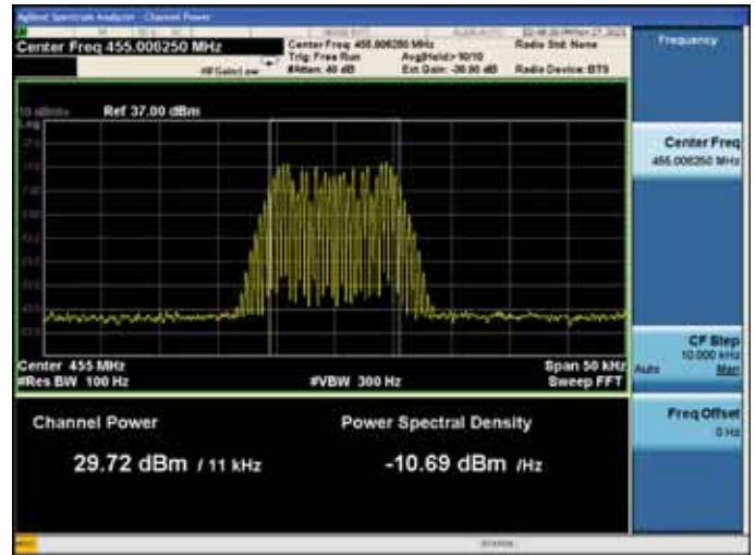
With the input signal amplitude set the AGC threshold Low Frequency: 455.00625MHz
