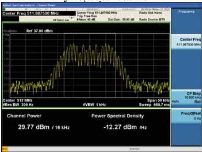
With the input signal amplitude set 3 dB above the AGC threshold High Frequency: 511.9875MHz
