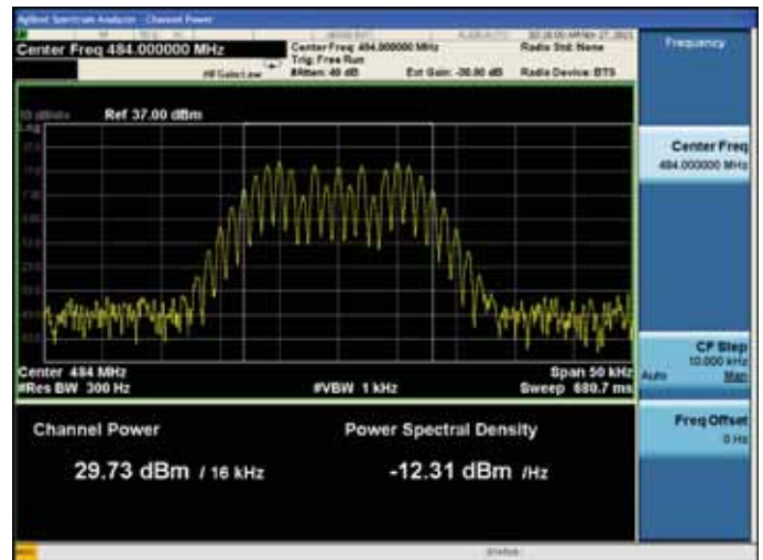
With the input signal amplitude set the AGC threshold Middle Frequency: 484.0MHz
