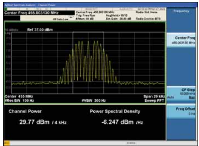
With the input signal amplitude set the AGC threshold Low Frequency: 455.00313MHz
