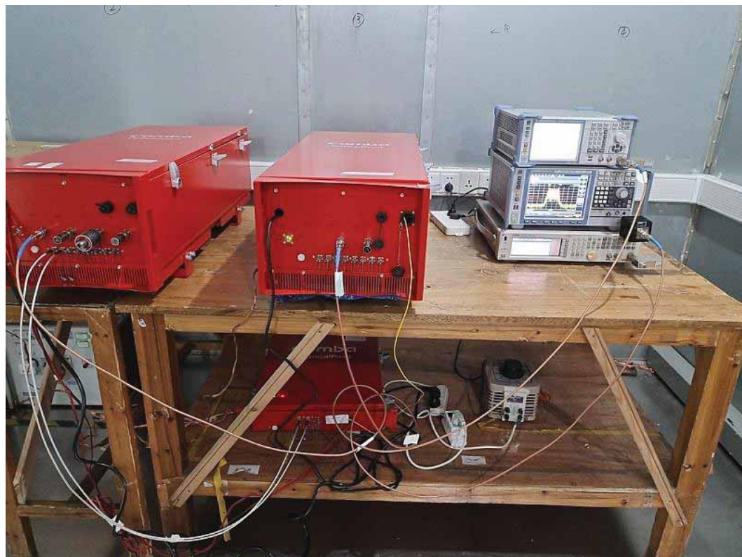
Normal temperature test scenario (AC power supply)
