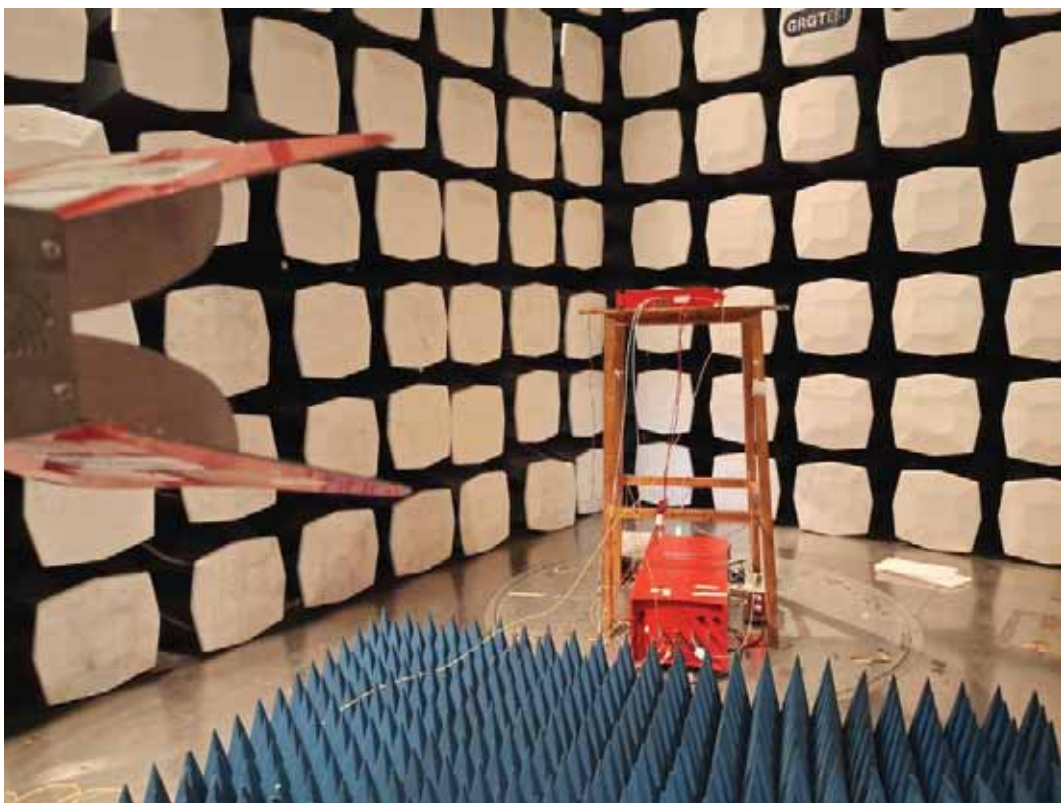
MU+FOU Radiated spurious emissions—Above 1GHz
