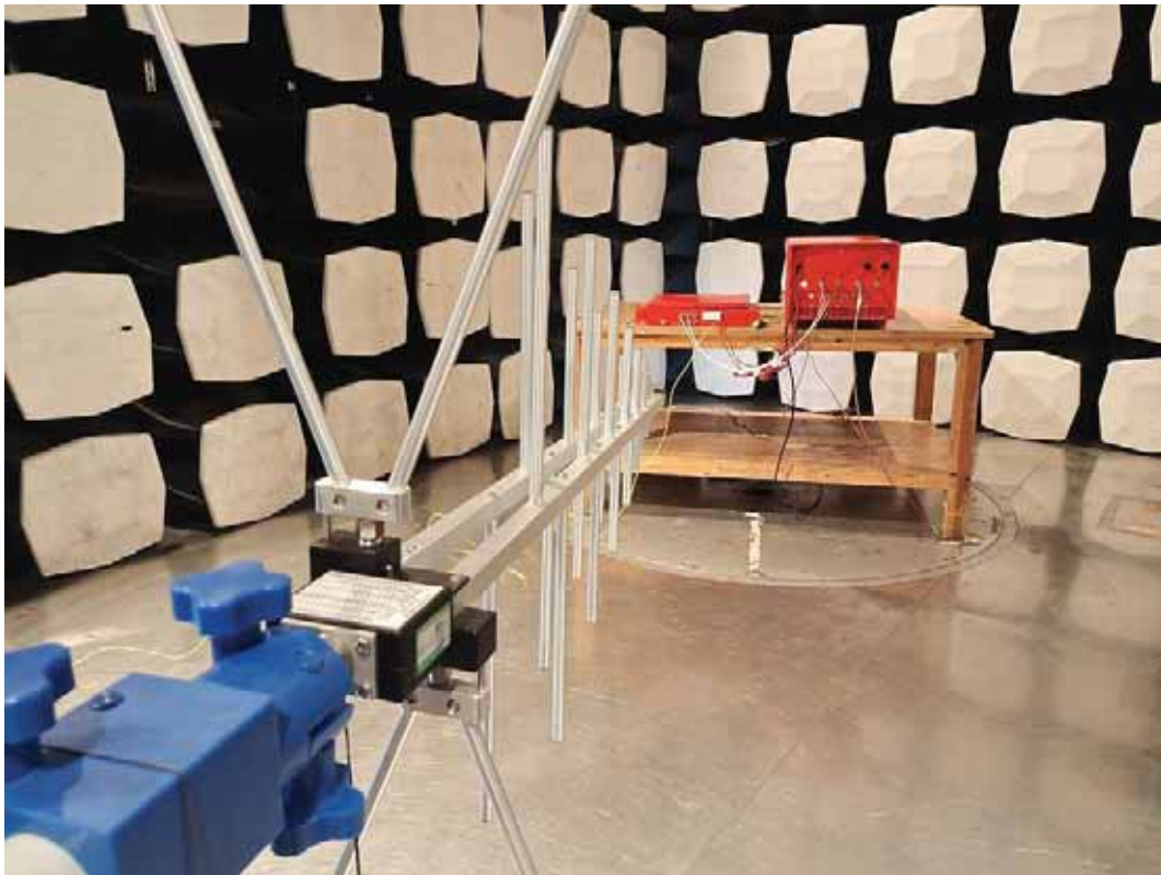
MU +FOU Radiated spurious emissions—Below 1GHz
