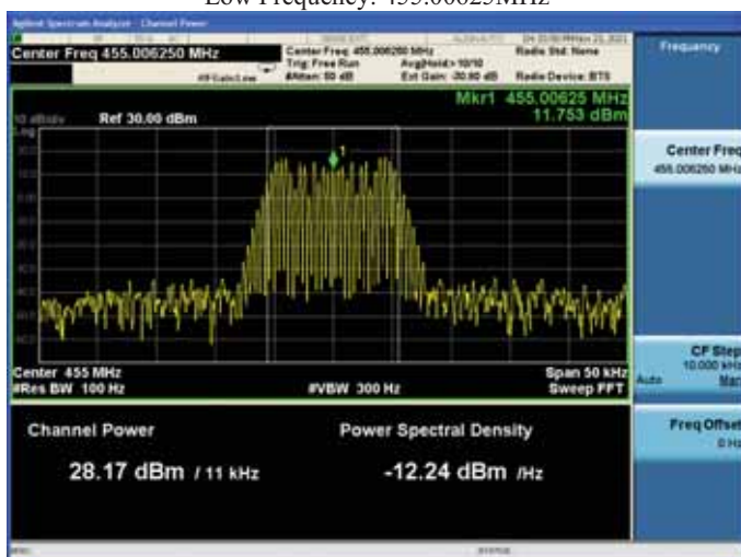
With the input signal amplitude set 3 dB above the AGC threshold Low Frequency: 455.00625MHz
