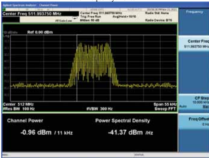
Input signal High Frequency: 511.99375MHz
