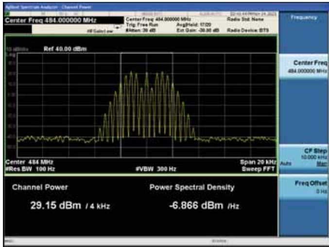
With the input signal amplitude set 3 dB above the AGC threshold Middle Frequency: 484.0MHz
