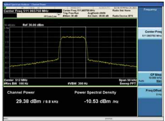
With the input signal amplitude set the AGC threshold High Frequency: 511.99375MHz
