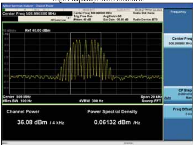
With the input signal amplitude set 3 dB above the AGC threshold High Frequency: 508.99688MHz
