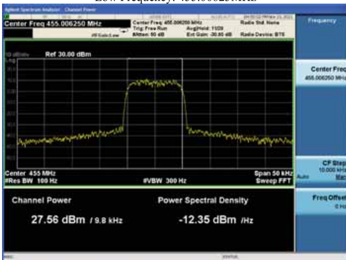
With the input signal amplitude set 3 dB above the AGC threshold
