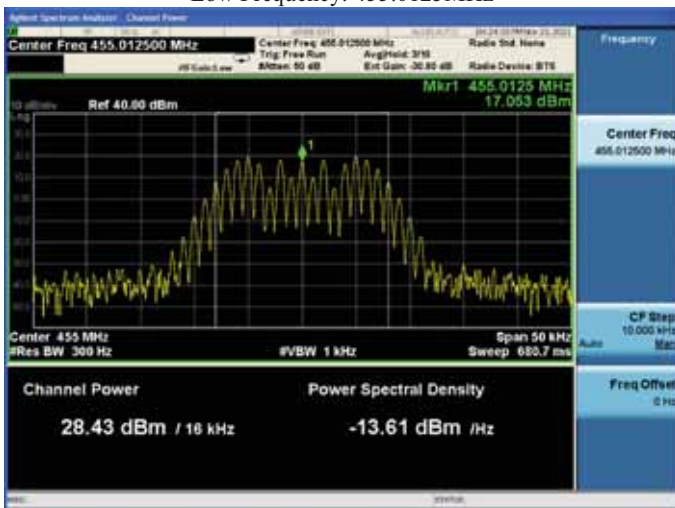
With the input signal amplitude set 3 dB above the AGC threshold Low Frequency: 455.0125MHz
