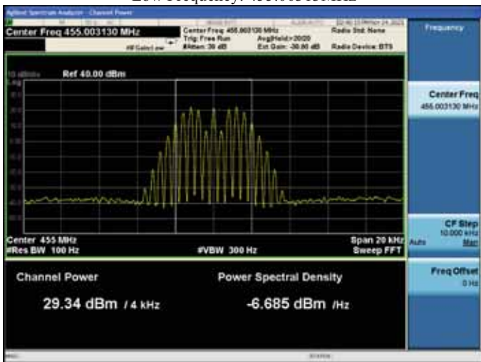
With the input signal amplitude set 3 dB above the AGC threshold Low Frequency: 455.00313MHz
