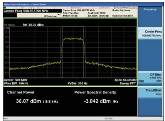
With the input signal amplitude set the AGC threshold High Frequency: 508.99375MHz
