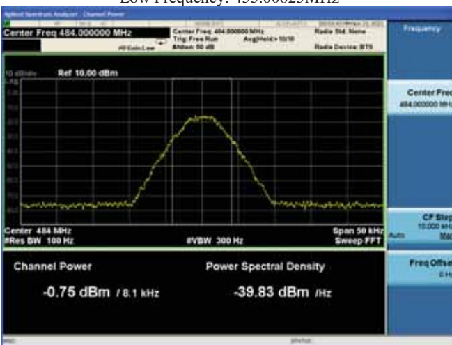
Input signal Middle Frequency: 484.0MHz
