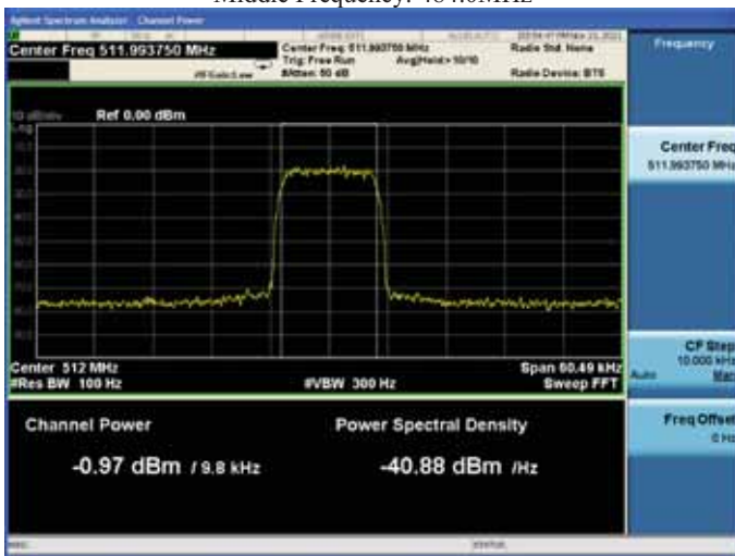
Input signal High Frequency: 511.99375MHz
