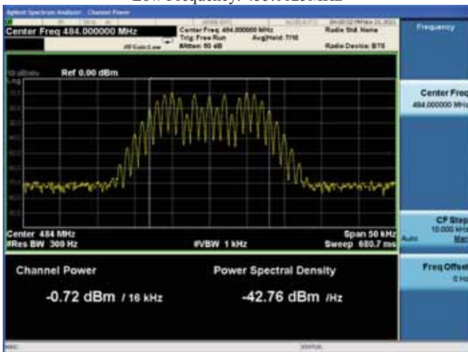
Input signal Middle Frequency: 484.0MHz
