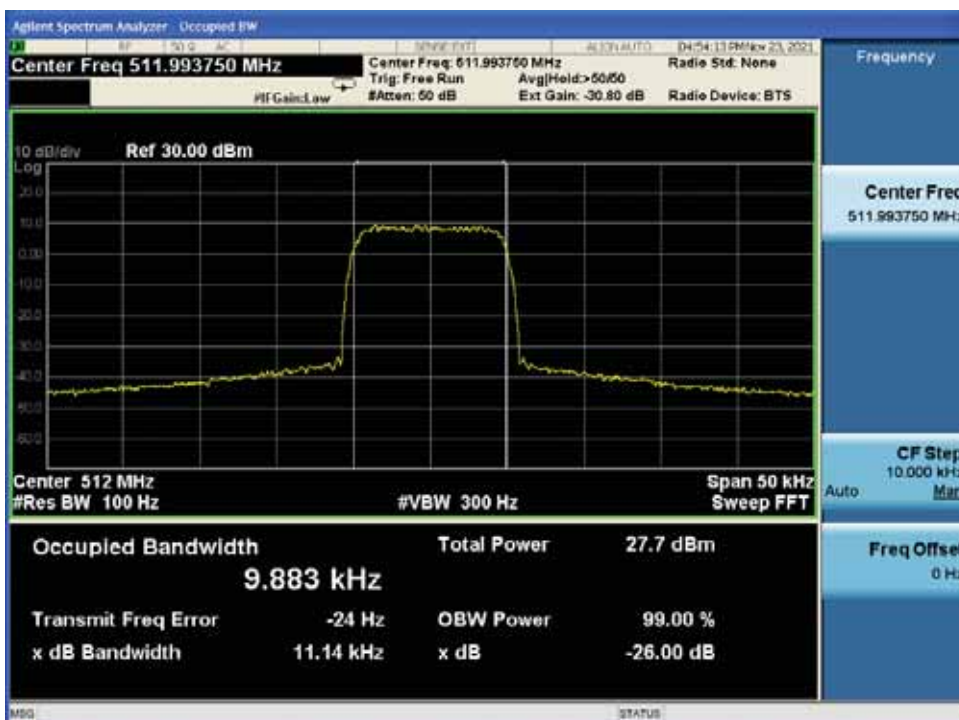
With the input signal amplitude set 3 dB above the AGC threshold High Frequency: 511.99375MHz
