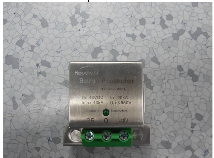
DC Surge protector
