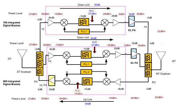
System gain: Downlink: 90dB; Uplink: 90dB.
