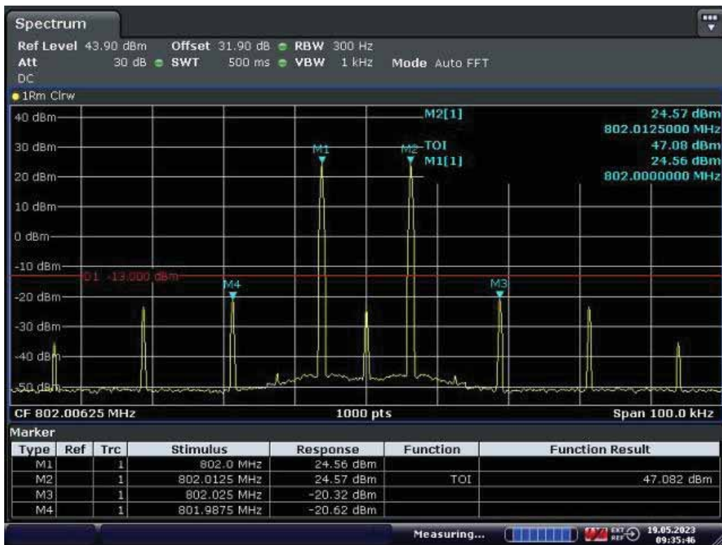
Mid Frequency and with the input signal amplitude set 3 dB above the ALC threshold
