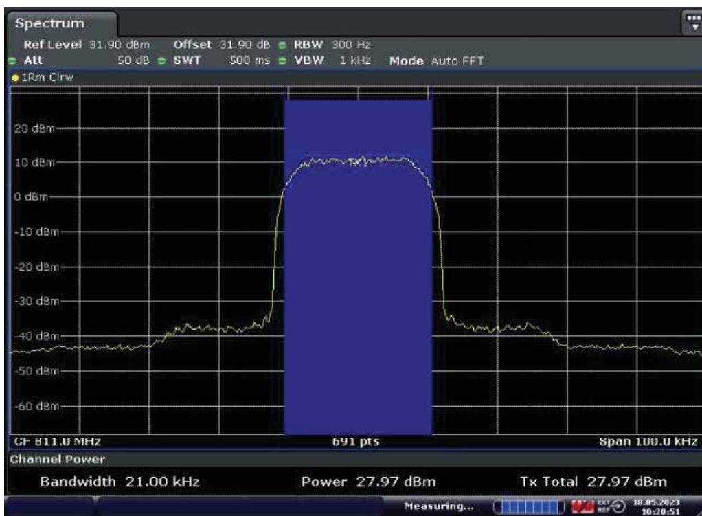
Middle Frequency: 811.0MHz, Output occupied BW (with the input signal amplitude set 3 dB above the AGC threshold)
