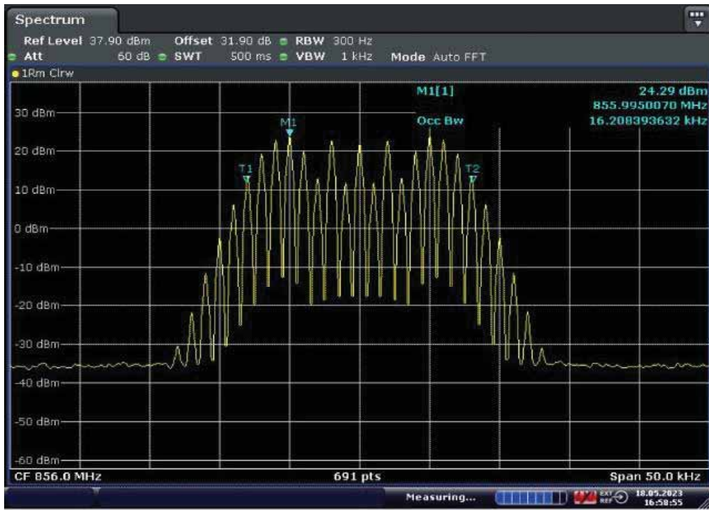
Middle Frequency: 856.0MHz, Output occupied BW (with the input signal amplitude set 3 dB above the AGC threshold)
