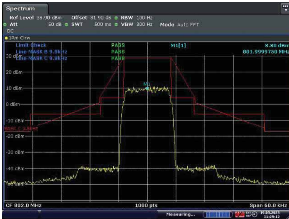
With the input signal amplitude set the AGC threshold Middle Frequency: 802.0MHz
