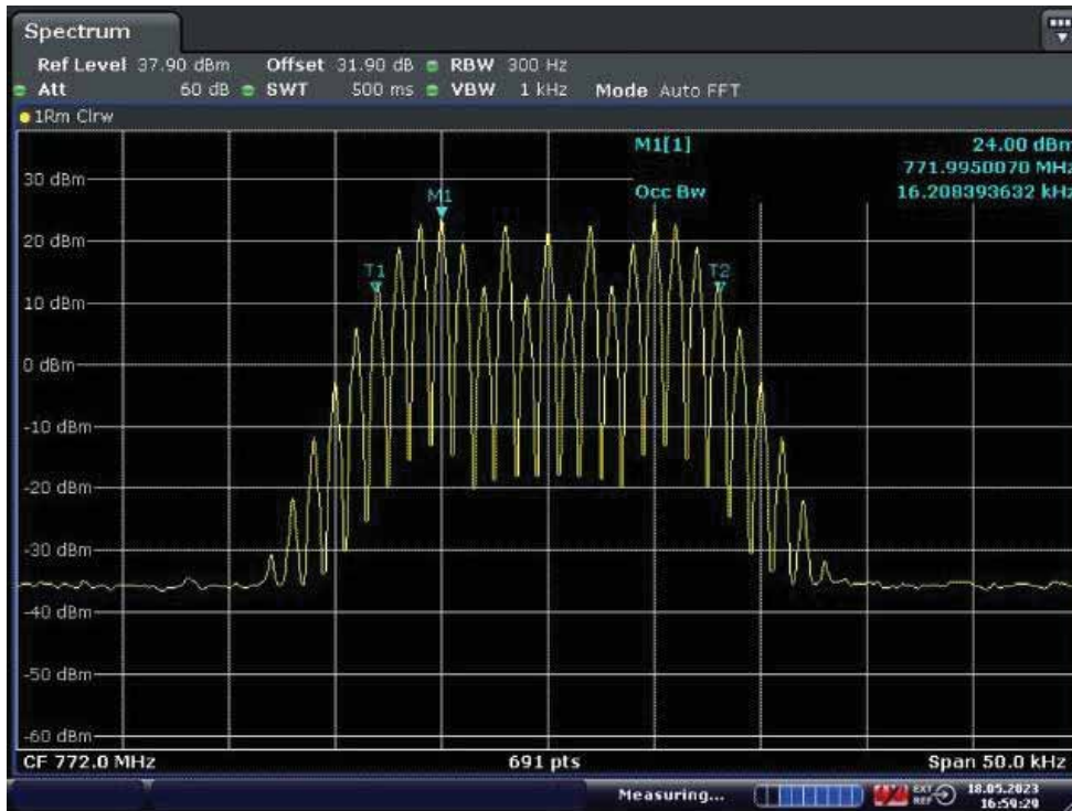
Middle Frequency: 772.0MHz, Output occupied BW(AGC)
