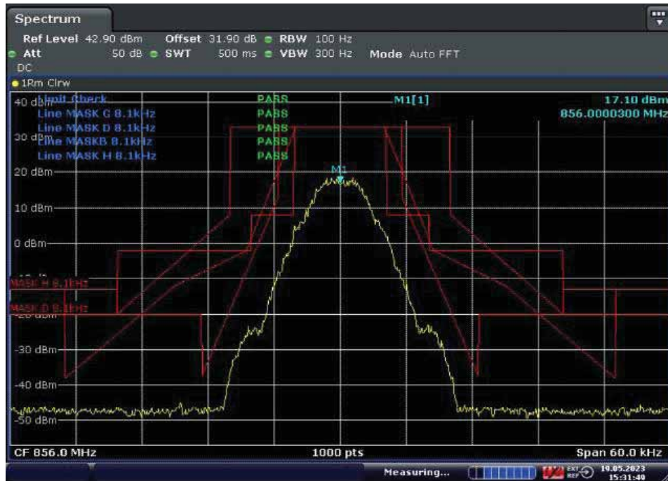
With the input signal amplitude set the AGC threshold Middle Frequency: 856.0MHz
