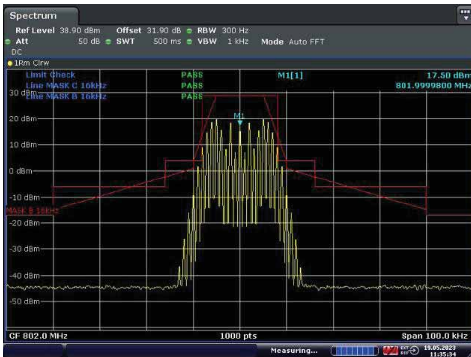
With the input signal amplitude set 3 dB above the AGC threshold Middle Frequency: 802.0MHz
