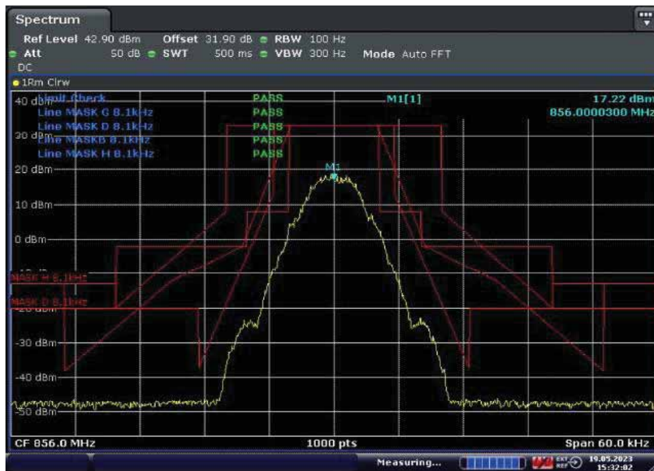
With the input signal amplitude set 3 dB above the AGC threshold Middle Frequency: 856.0MHz
