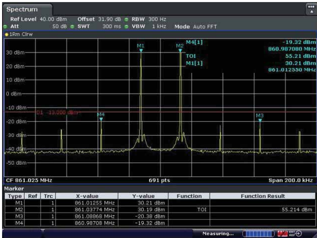
Low Frequency and with the input signal amplitude set 3 dB above the ALC threshold
