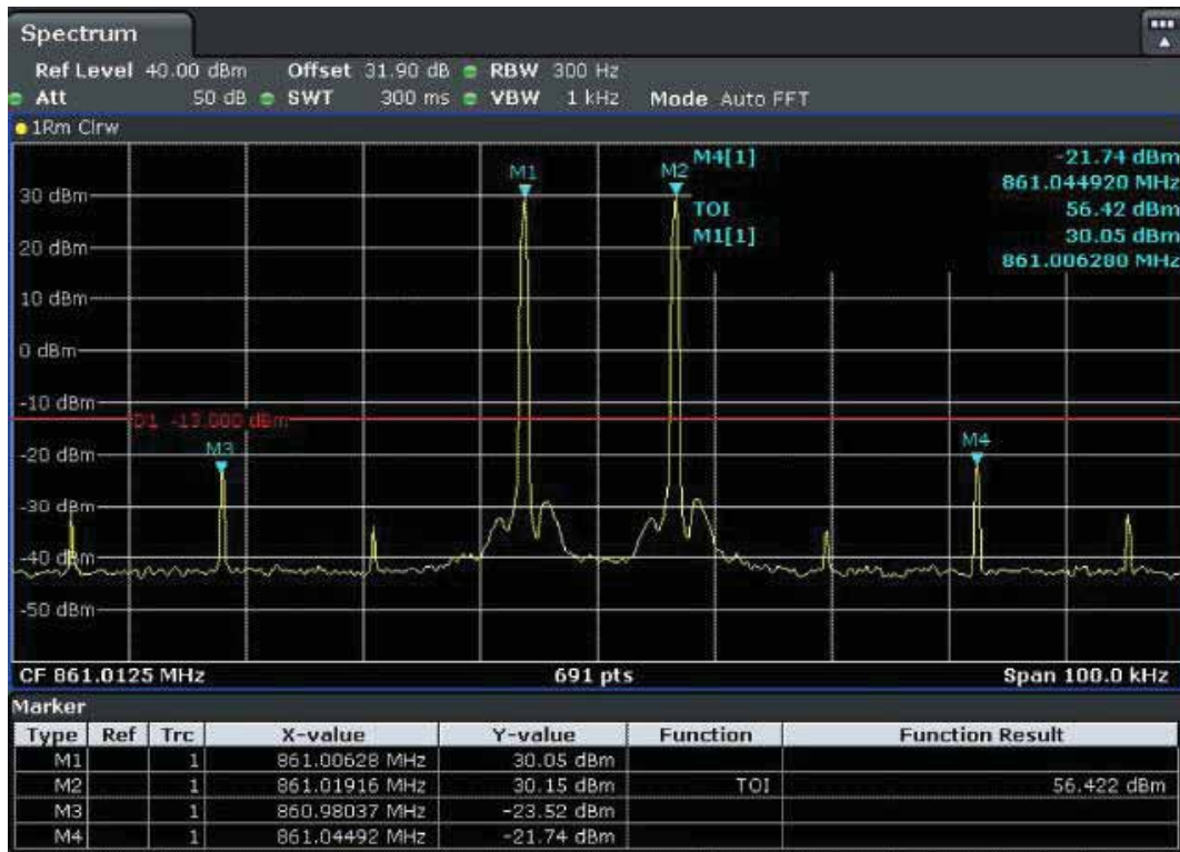
Low Frequency and with the input signal amplitude set 3 dB above the ALC threshold
