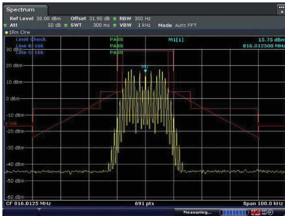
With the input signal amplitude set 3 dB above the AGC threshold Lowest Frequency: 816.0125MHz
