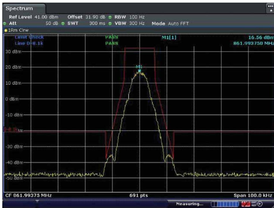
With the input signal amplitude set 3 dB above the AGC threshold Highest Frequency: 861.99375MHz
