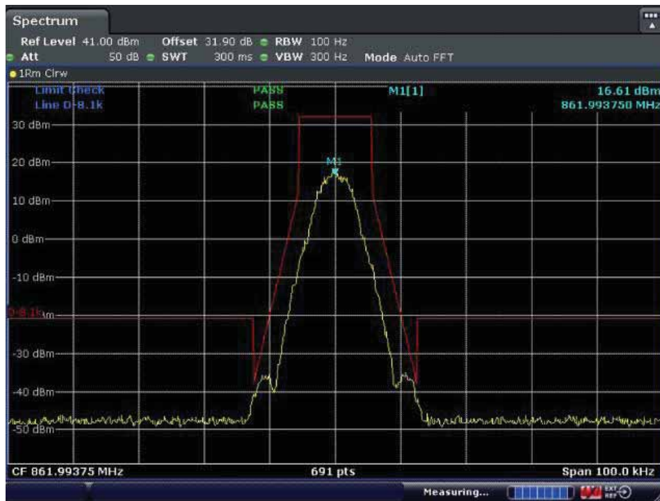
With the input signal amplitude set the AGC threshold Highest Frequency: 861.99375MHz
