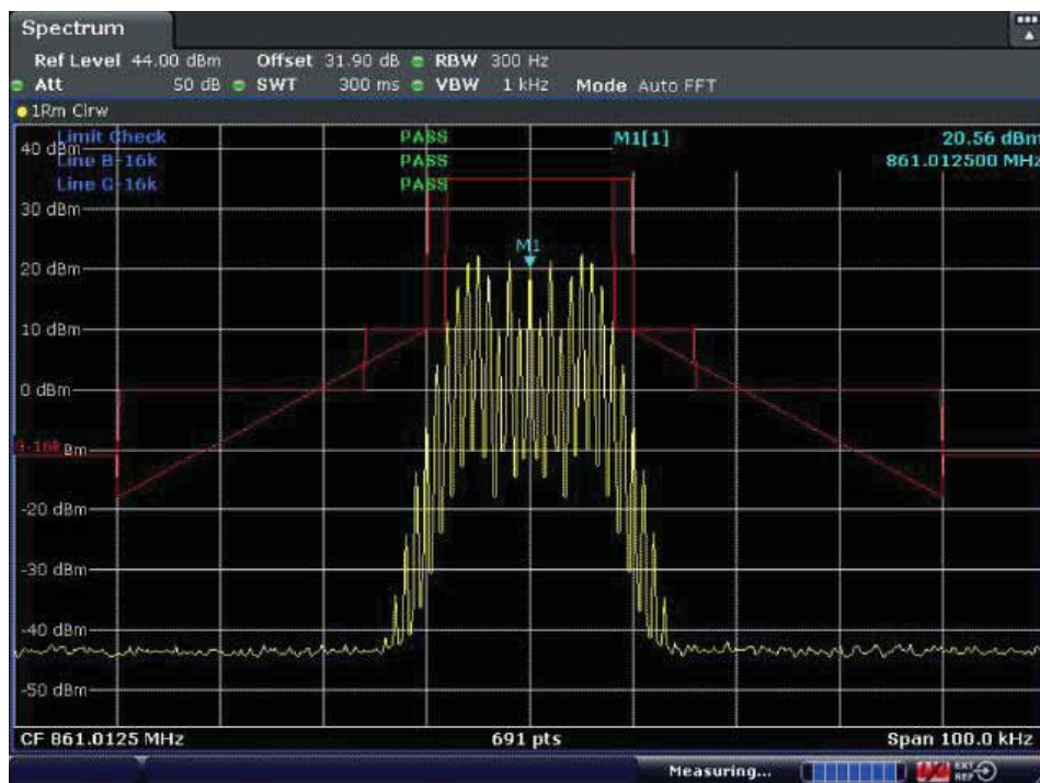
With the input signal amplitude set 3 dB above the AGC threshold Lowest Frequency: 861.0125MHz
