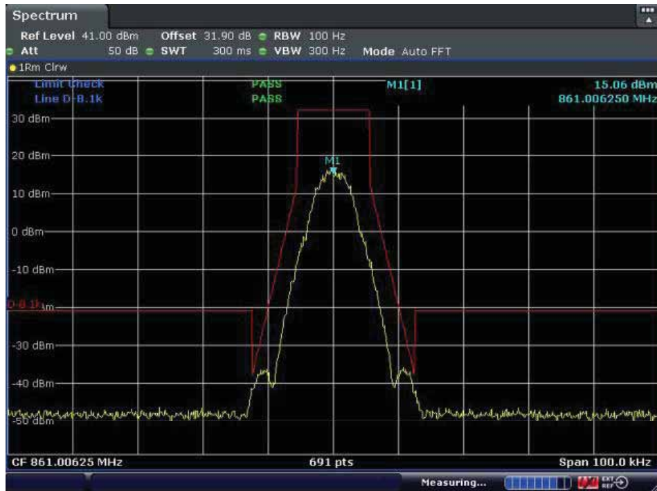
With the input signal amplitude set the AGC threshold Lowest Frequency: 861.00625MHz
