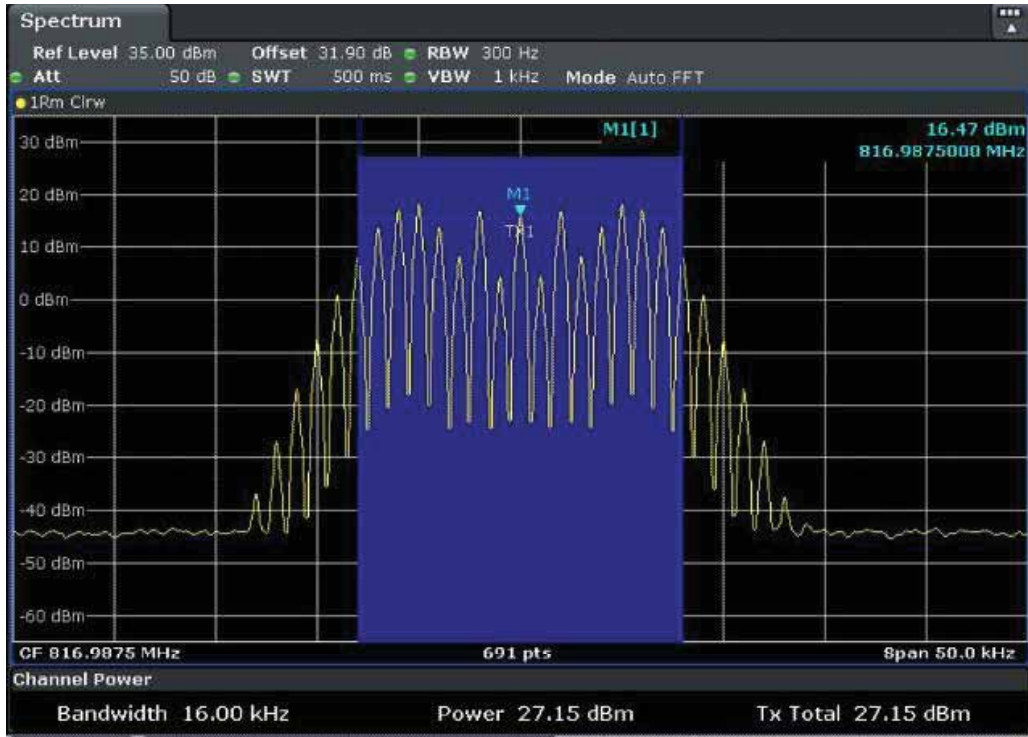
Highest Frequency: 816.9875MHz, Output occupied BW(AGC)
