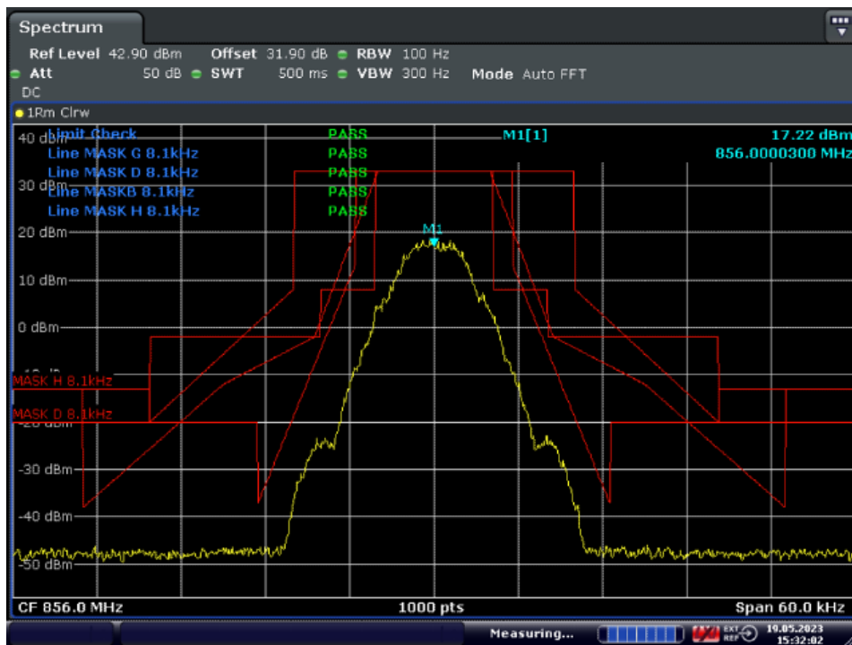
With the input signal amplitude set 3 dB above the AGC threshold Middle Frequency: 856.0MHz
