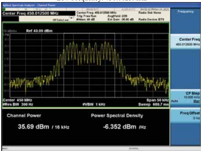
With the input signal amplitude set 3 dB above the AGC threshold Low Frequency: 450.0125MHz
