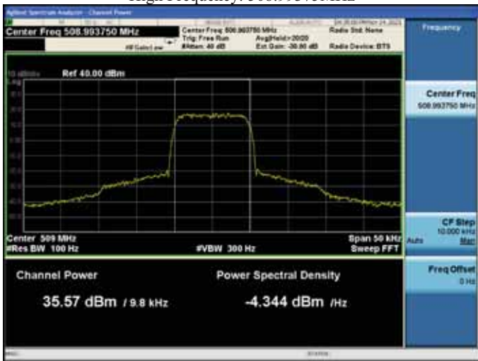
With the input signal amplitude set 3 dB above the AGC threshold High Frequency: 508.99375MHz
