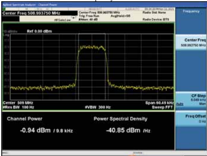
Input signal High Frequency: 508.99375MHz
