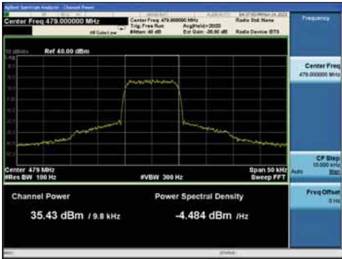
With the input signal amplitude set 3 dB above the AGC threshold Middle Frequency: 479.0MHz
