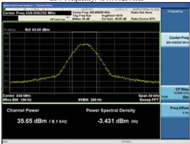
With the input signal amplitude set 3 dB above the AGC threshold Low Frequency: 450.00625MHz
