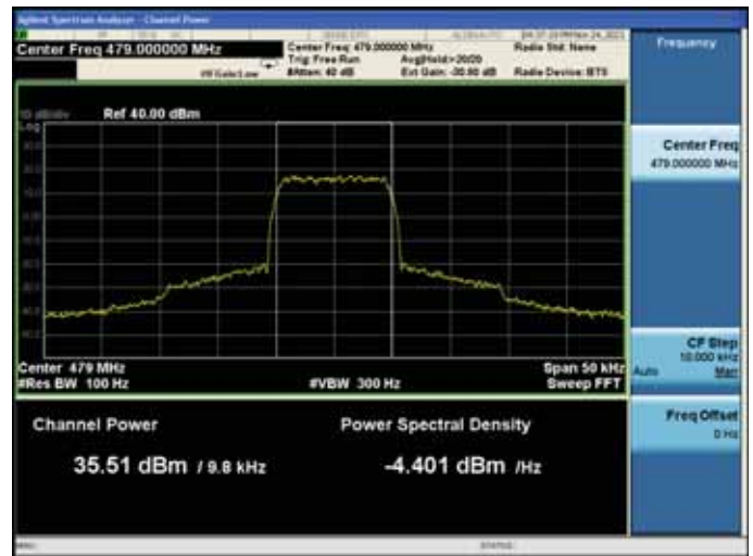
With the input signal amplitude set the AGC threshold Middle Frequency: 479.0MHz
