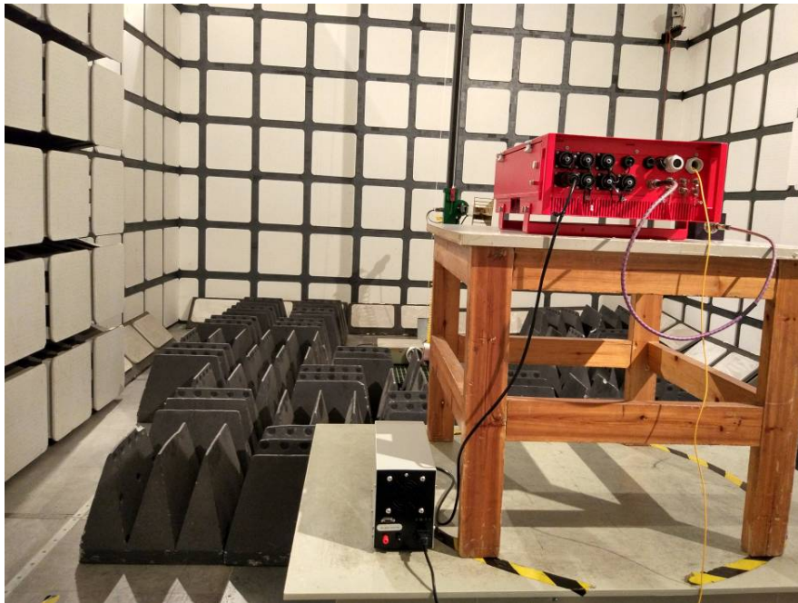
Transmitting Radiated Emissions Tested – Rear View (Above 1 GHz)
