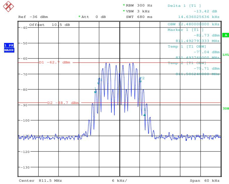
**Frequency: 811.5 MHz, 99% Occupied & 26 dB Bandwidth AGC+3 Output**
