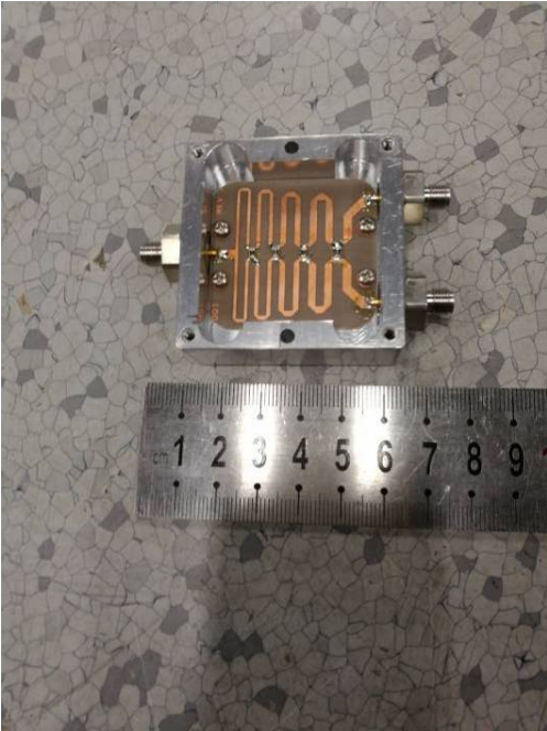
EUT – Splitter Module 3 Board View
