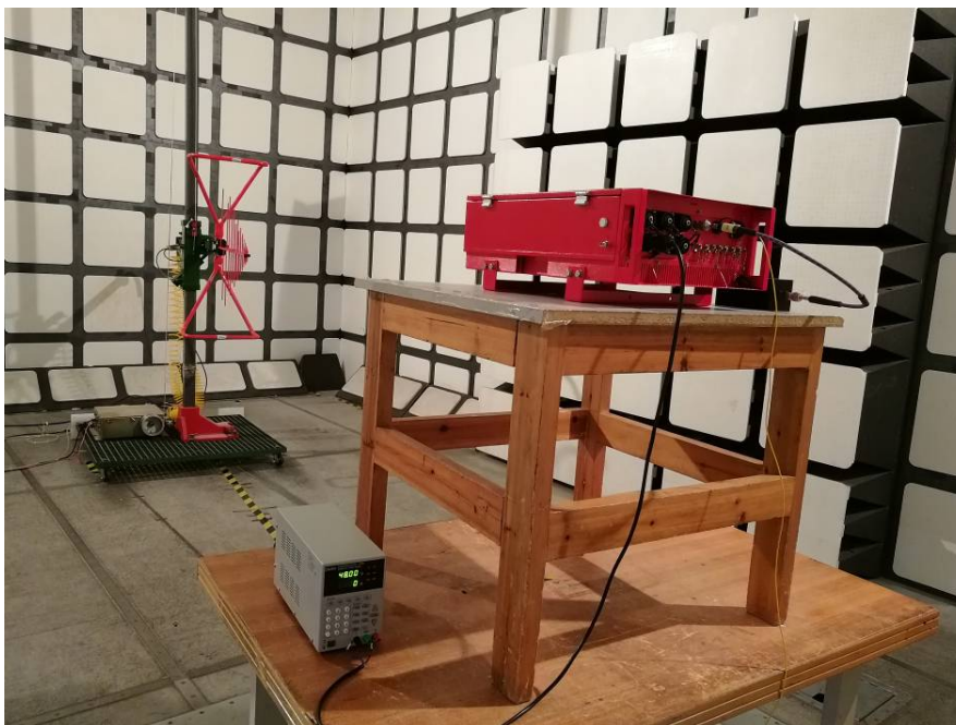
Transmitting Radiated Emissions Tested - Rear View (Below 1 GHz)
