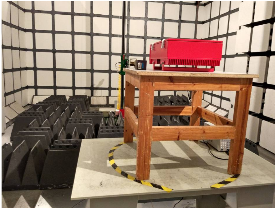
Transmitting Radiated Emissions Tested – Front View (Above 1 GHz)
