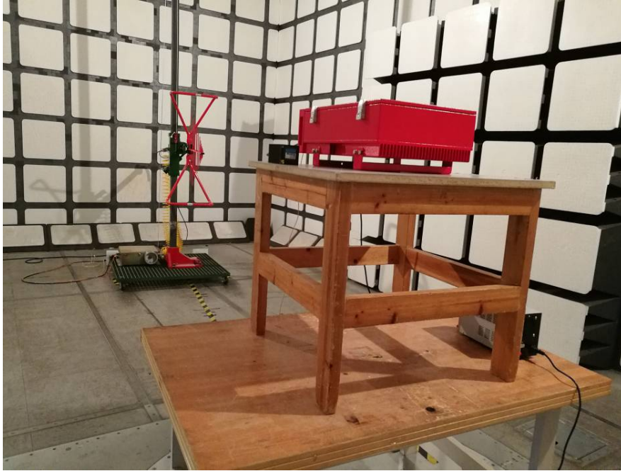
Transmitting Radiated Emissions Tested - Rear View (Below 1 GHz)
