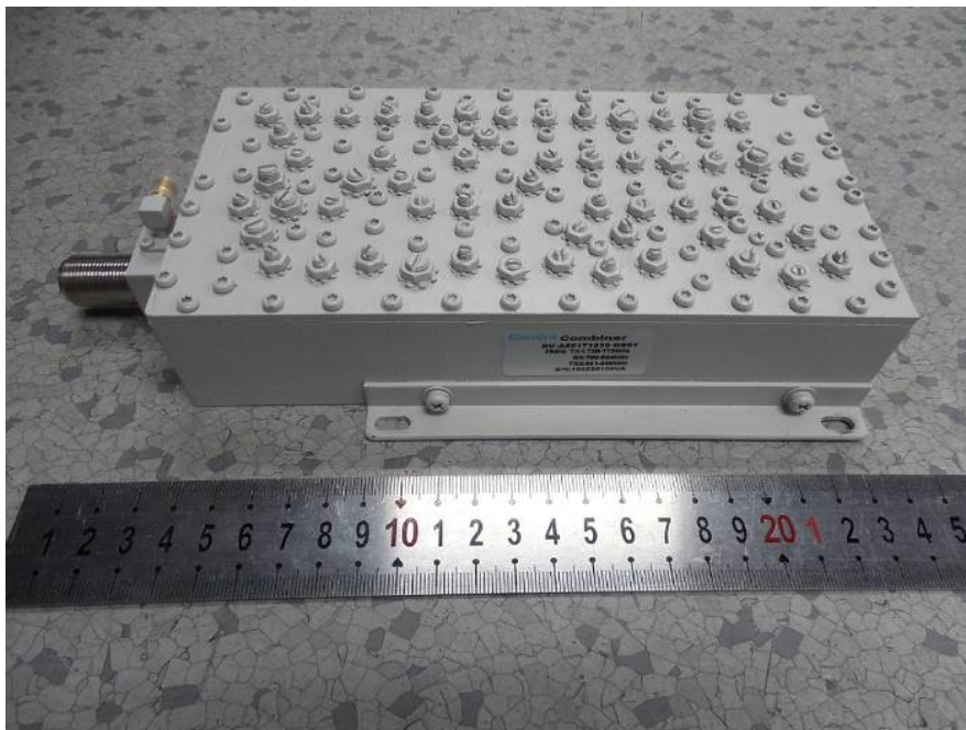
EUT – Duplexer Module View 1
