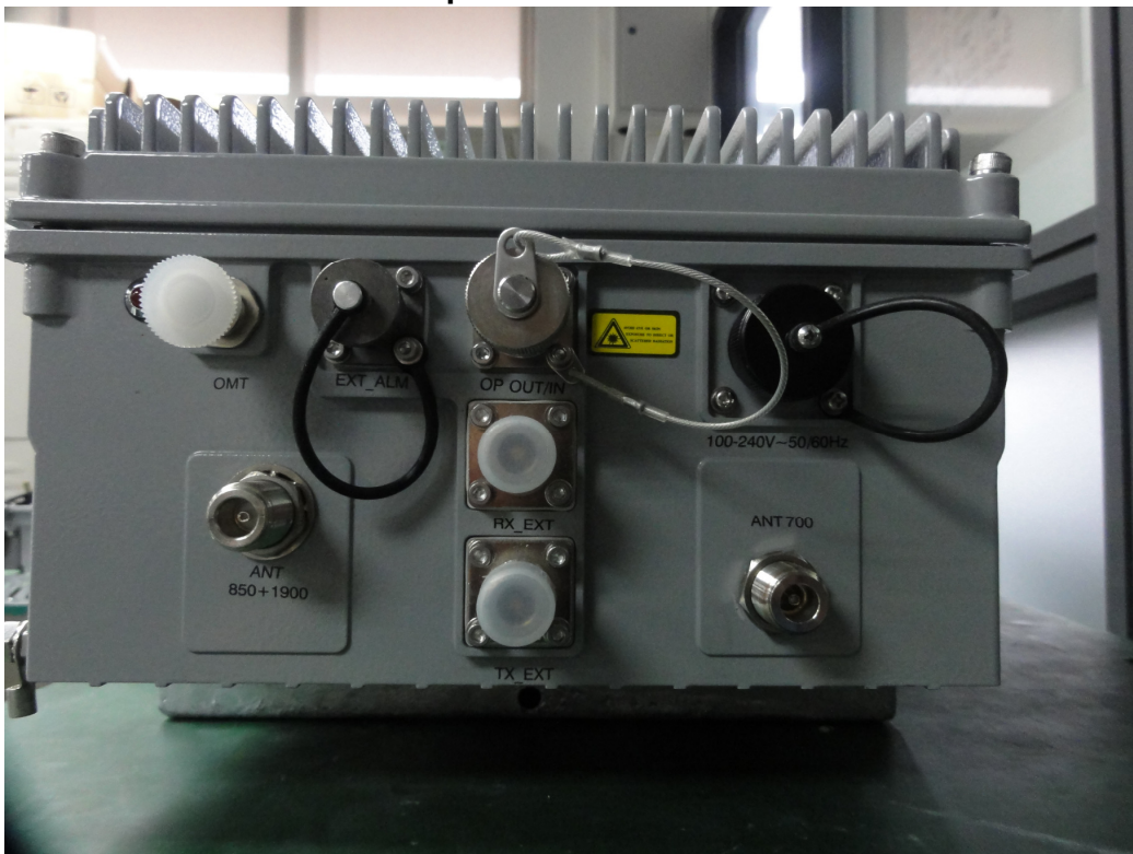
I/O port of Remote Unit
