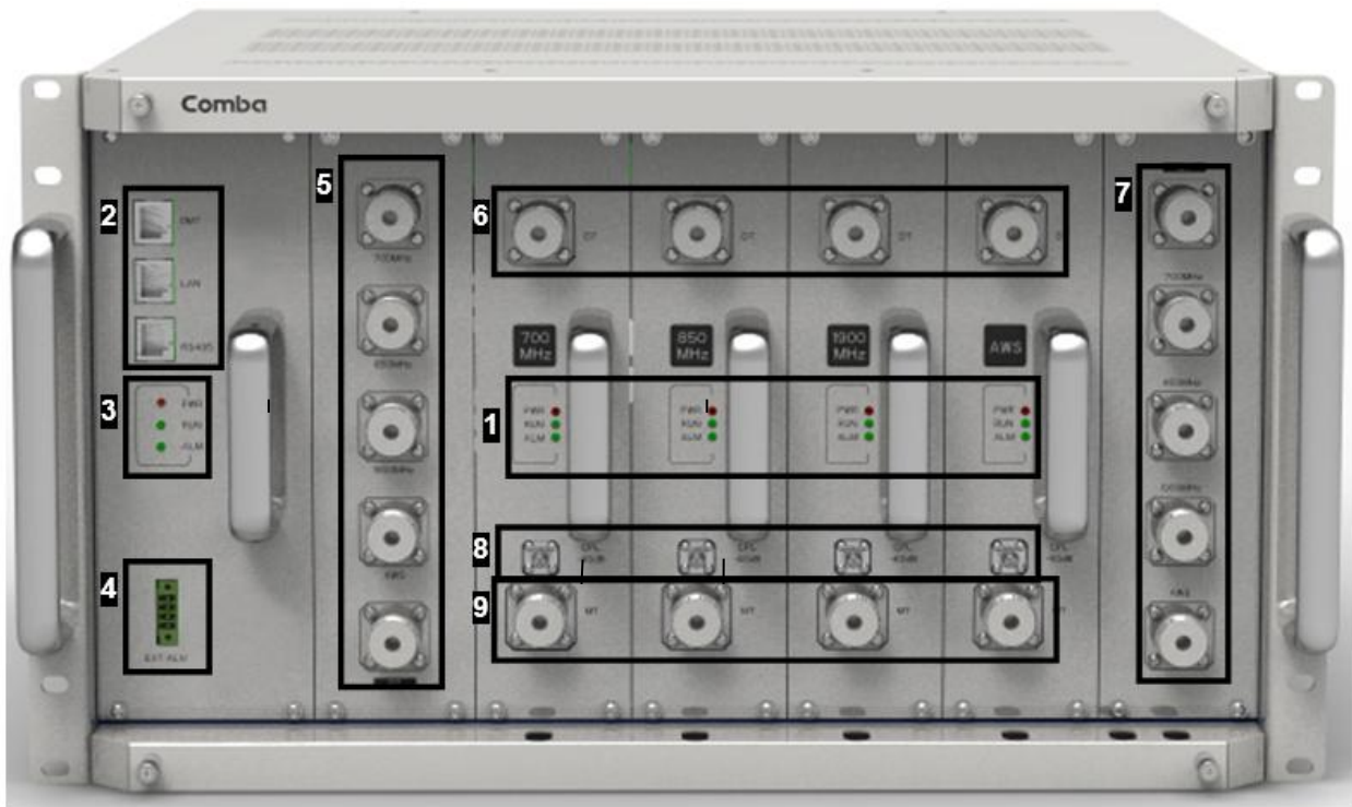
Figure 19: mBDA Front Panel Connectors
