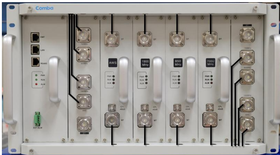
Figure 5: mBDA with 4 RFU and Combiners Configuration (example)
