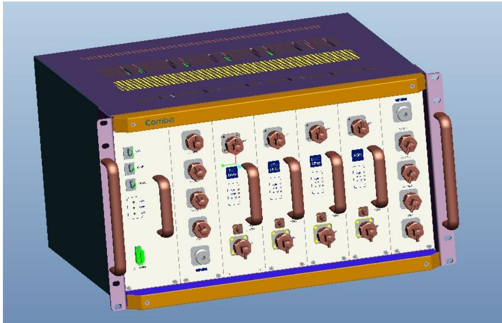
Figure 13: Completed mBDA of Four RFU and Two Combiners Installation
