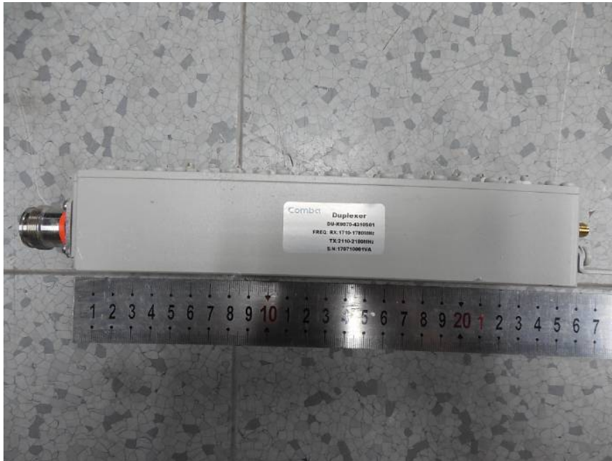
EUT –Duplexer side view
