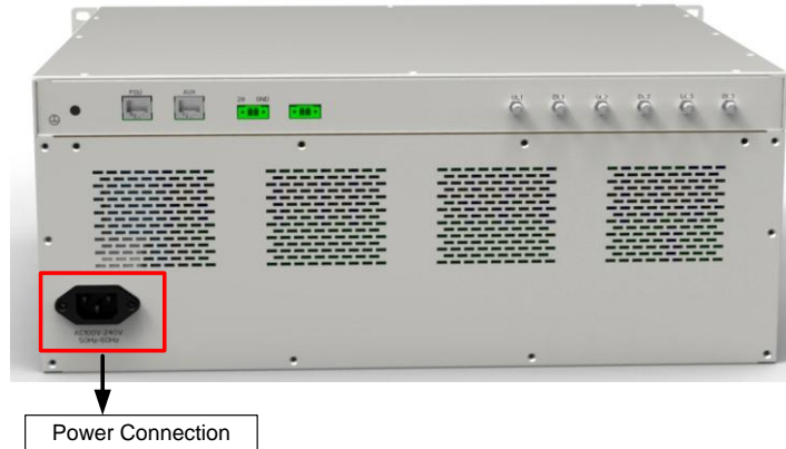
Figure 2: MU Power Connection (Rear Panel)
