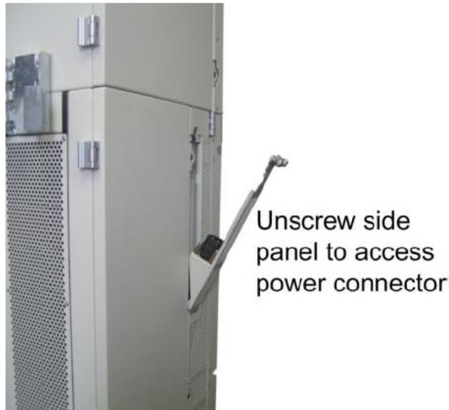
Figure 4: PSU Power Port Connection
