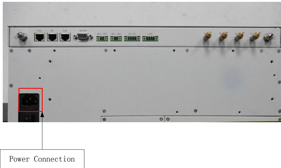
Figure 30: MU Power Connection (Rear Panel)
