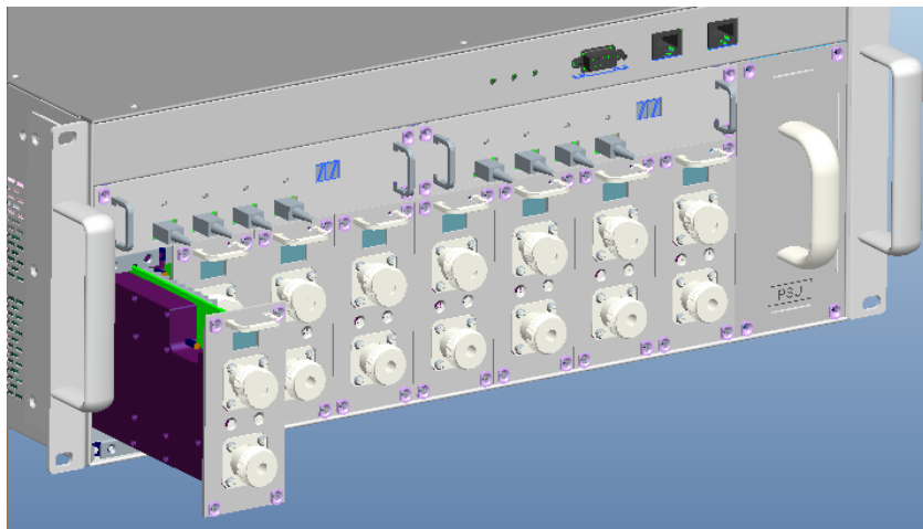
Figure 6: RF Unit Installation
