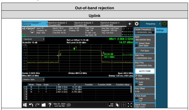
The peak of the frequency response f0 is 2566.3MHz. The frequency point f0 with the highest power level fall in the CMRS band under test, EUT is compiled the 935210 D05 Indus Booster Basic Meas v01r04 Out-of-band rejection verification test requirement.
