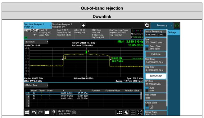
The peak of the frequency response f0 is 3839.3MHz. The frequency point f0 with the highest power level fall in the CMRS band under test, EUT is compiled the 935210 D05 Indus Booster Basic Meas v01r04 Out-of-band rejection verification test requirement.
