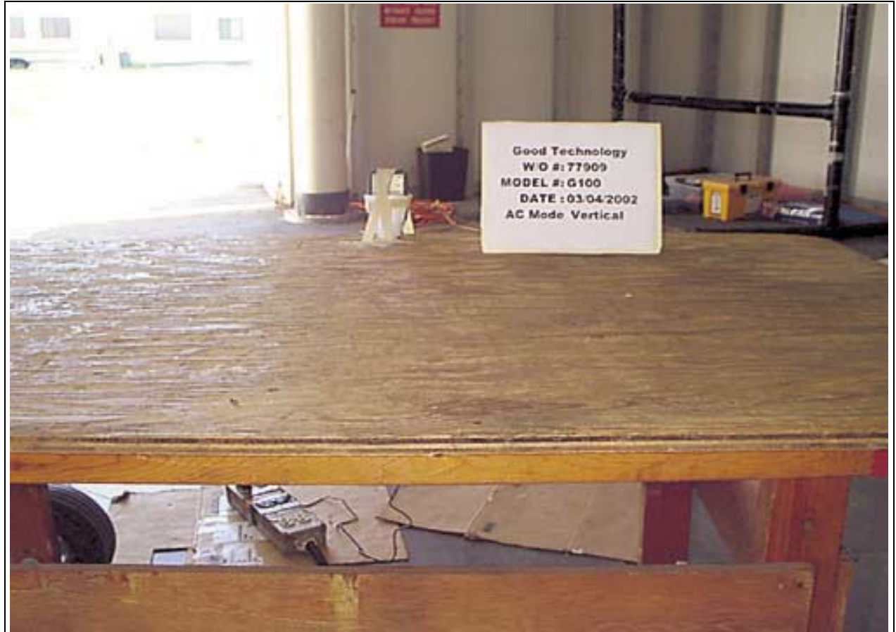
Radiated Emissions - Front View - AC Adapter Vertical
