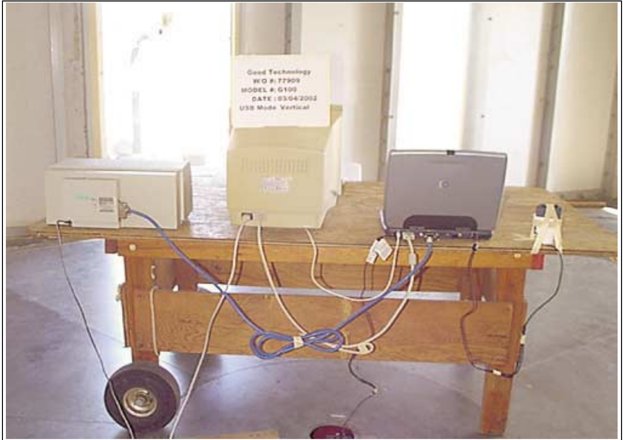
Radiated Emissions - Back View - USB Vertical
