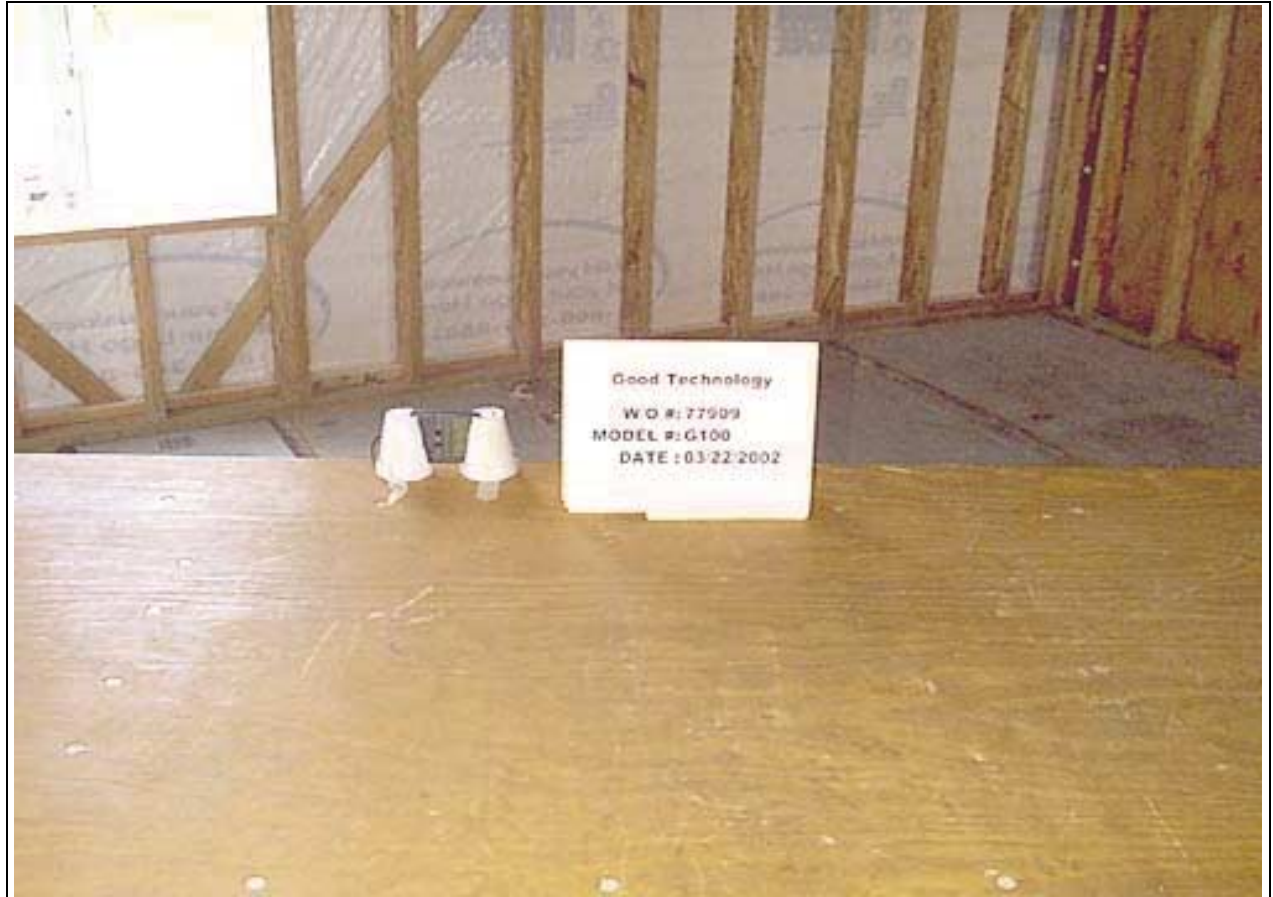
Radiated Emissions - Front View - AC Adapter Horizontal
