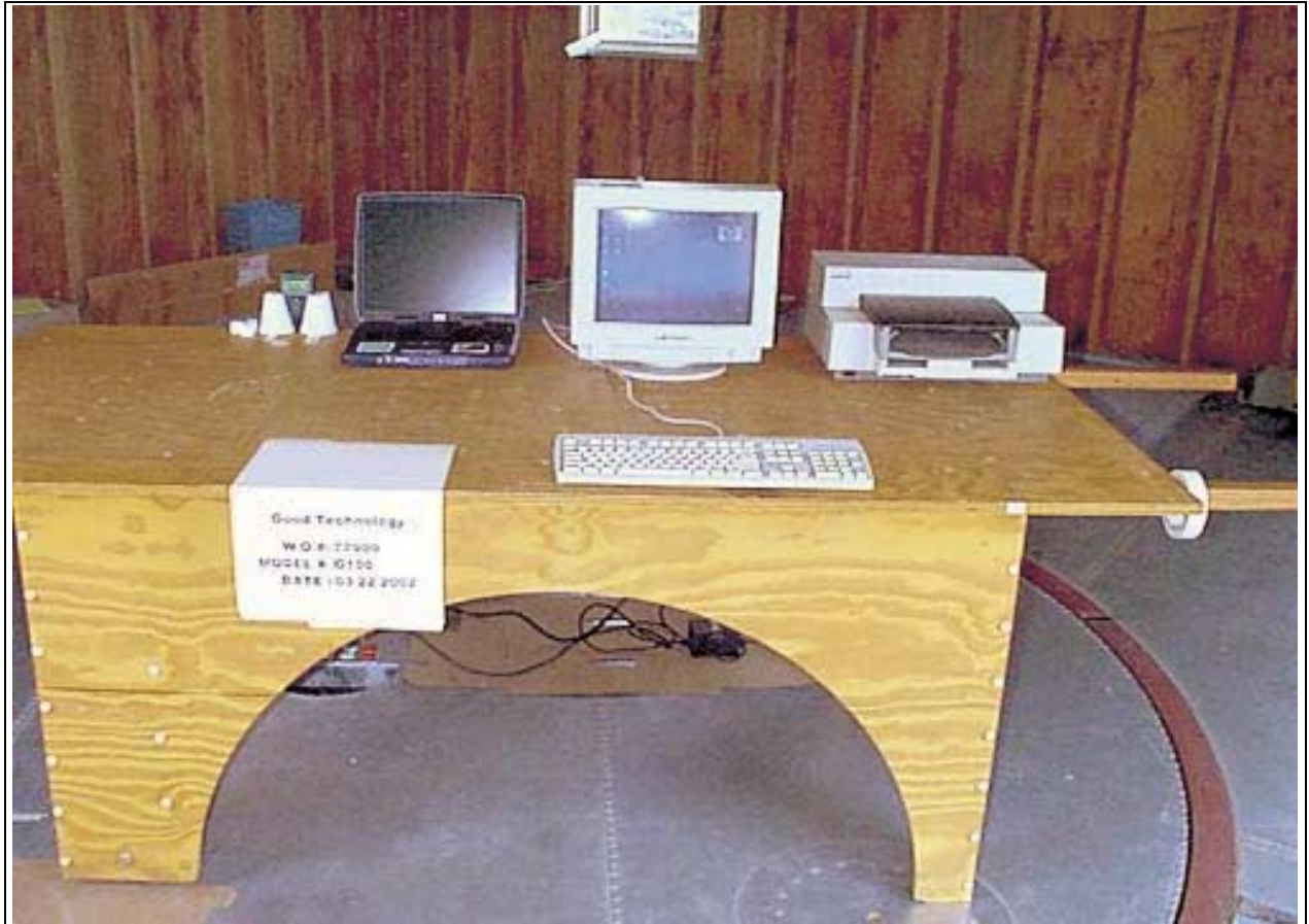
Radiated Emissions - Front View - USB Vertical
