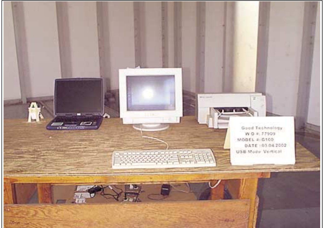
Radiated Emissions - Front View - USB Vertical
