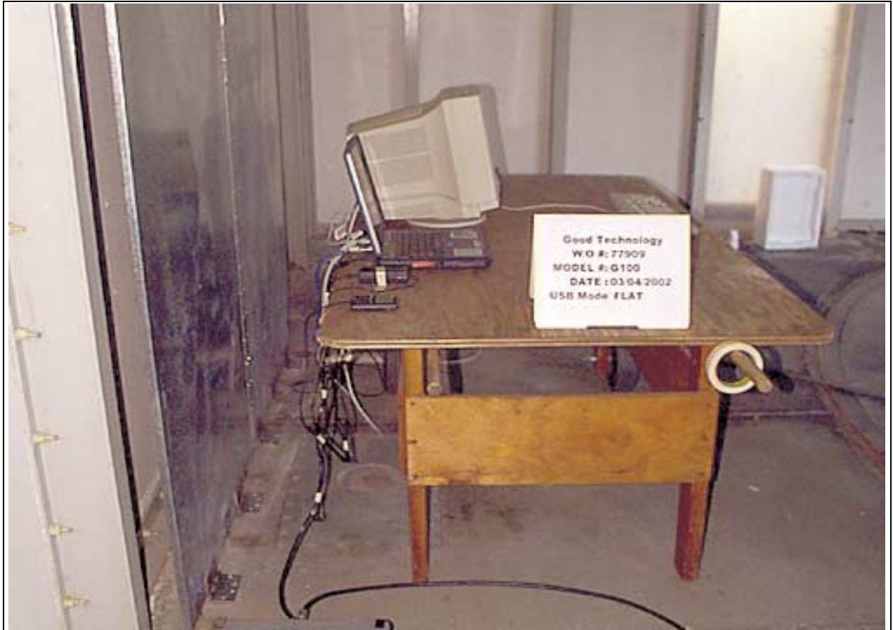
Mains Conducted Emissions - Side View - USB
