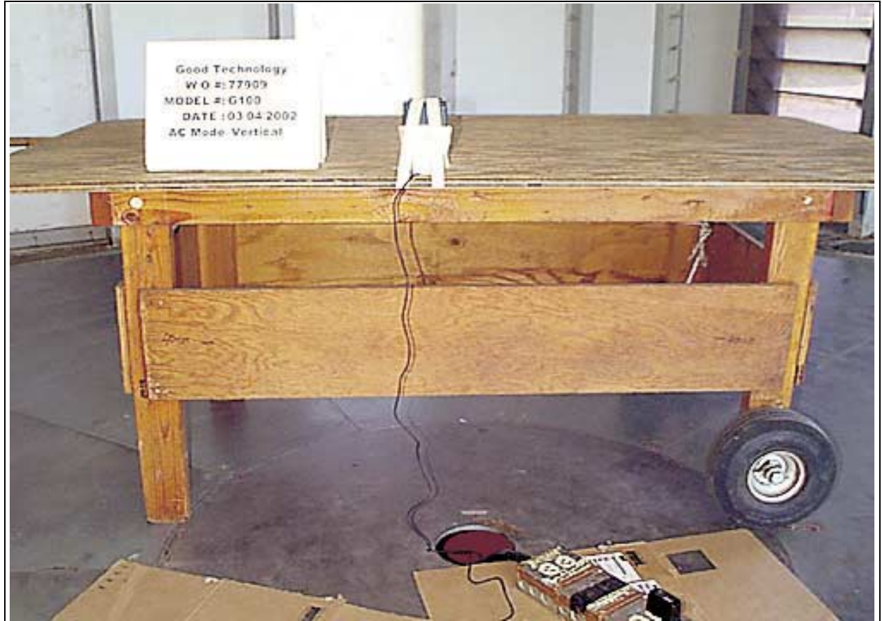
Radiated Emissions - Back View - AC Adapter Vertical
