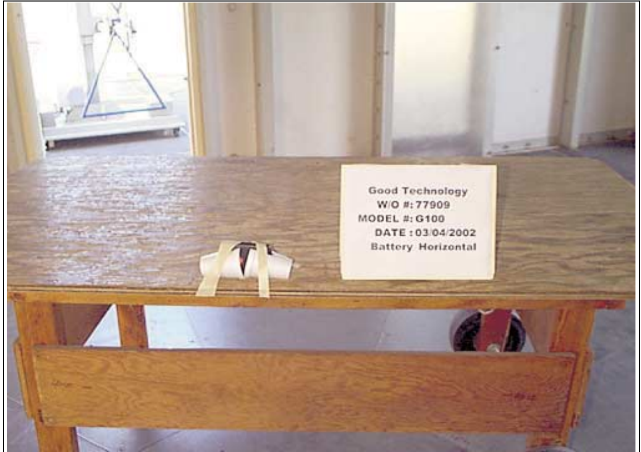
Radiated Emissions - Back View - Battery Horizontal
