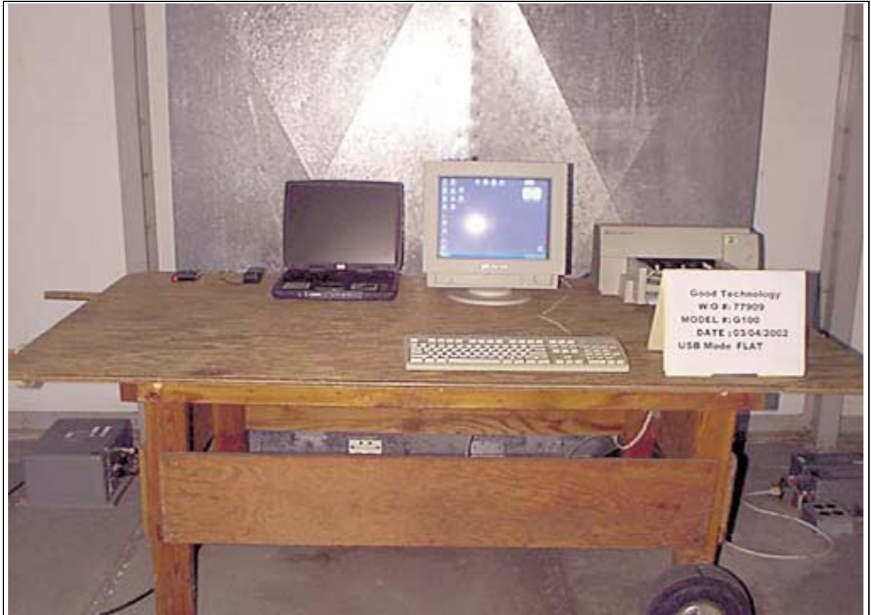
Mains Conducted Emissions - Front View - USB
