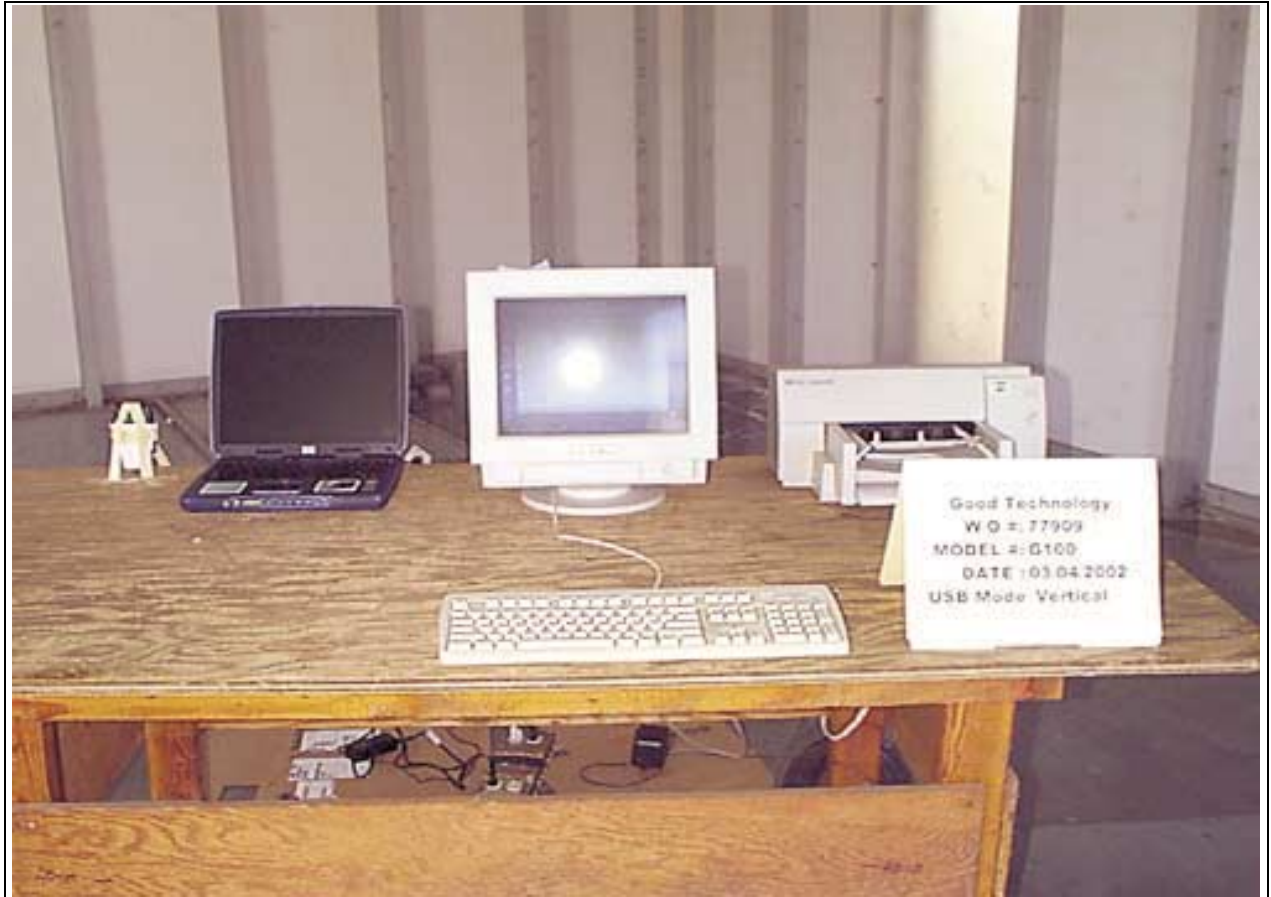
Radiated Emissions - Front View - USB Vertical
