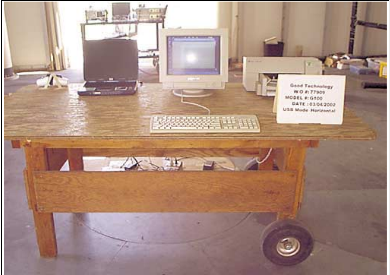
Radiated Emissions - Front View - USB Horizontal
