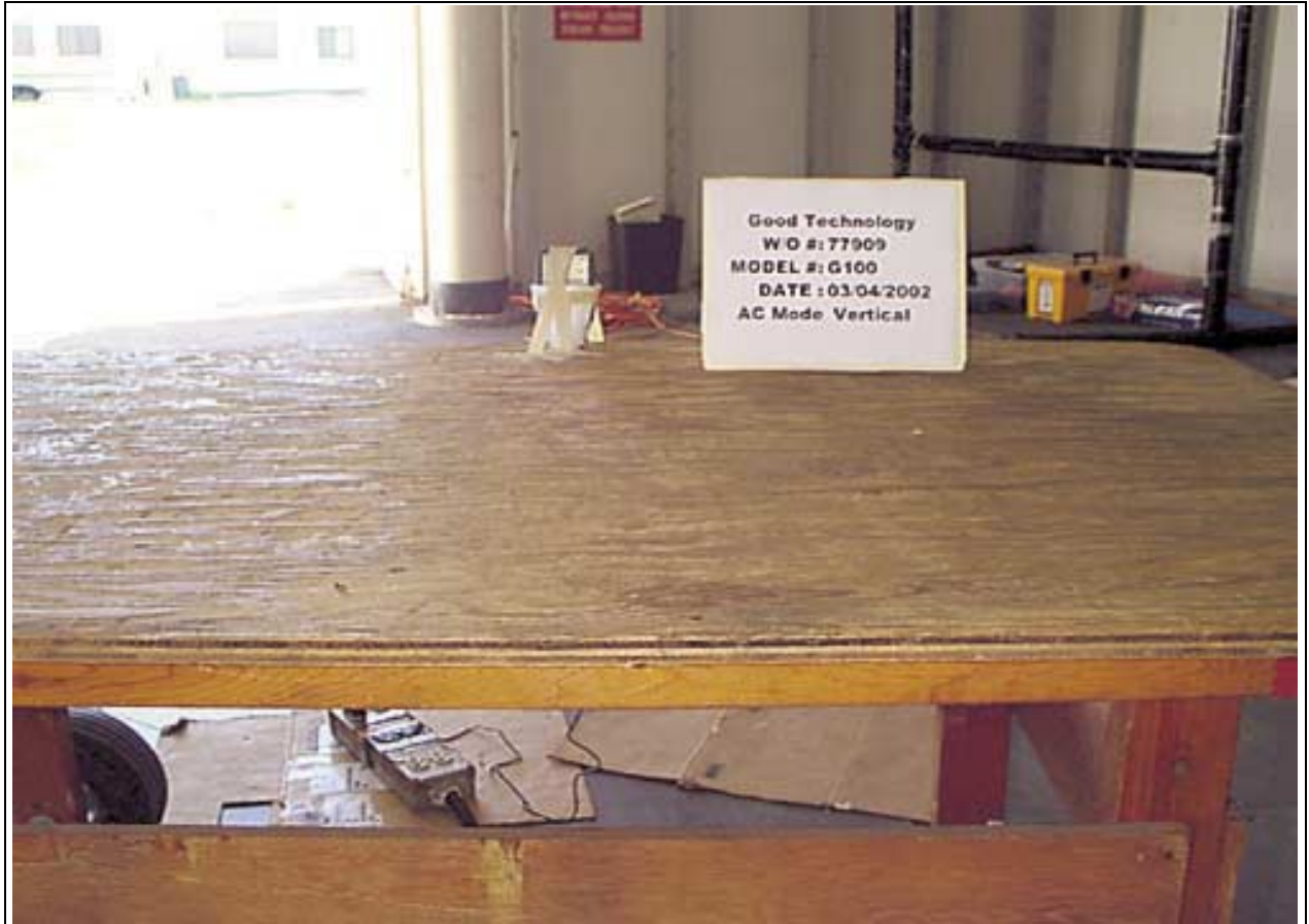
Radiated Emissions - Front View - AC Adapter Vertical
