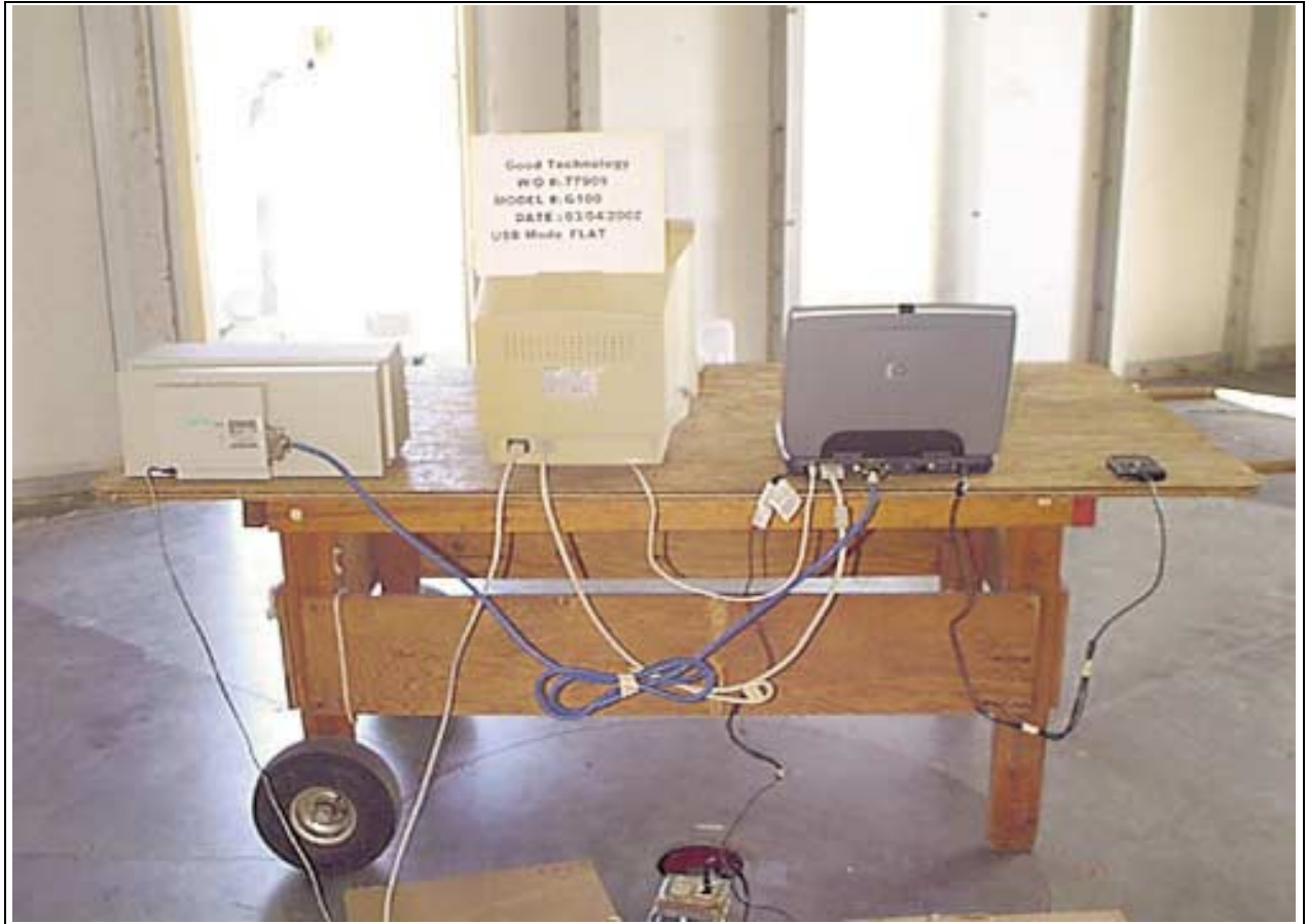
Radiated Emissions - Back View - USB Flat
