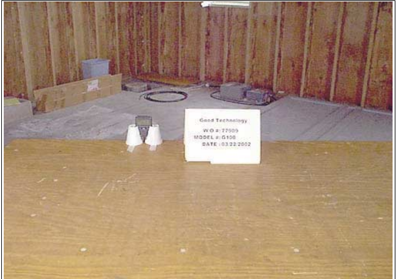
Radiated Emissions - Front View - AC Adapter Vertical
