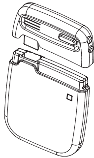
Figure 9. Connecting the EPG header to the EPG
