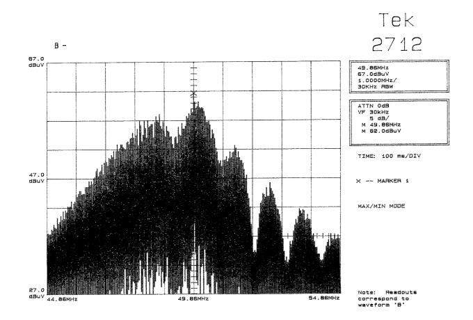
Note: A signal generator was set to the unit under test operating frequency. An unmodulated continuous wave (CW) signal was radiated at the superregenerative receiver operating frequency to cohere the characteristic broadband emissions from the receiver.
