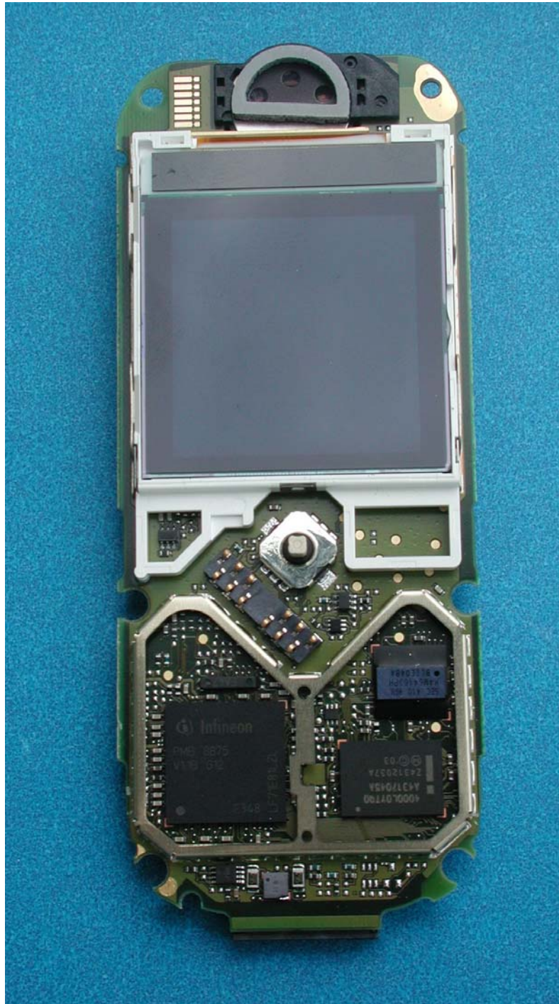
C65 PCB Front View Shields Removed
