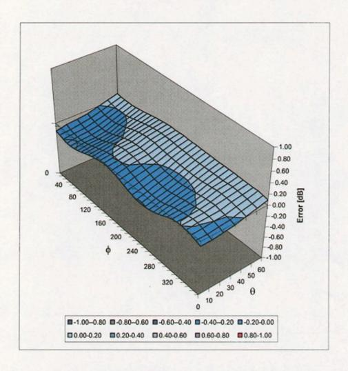
Spherical Isotropy Error < ± 0.4 dB
