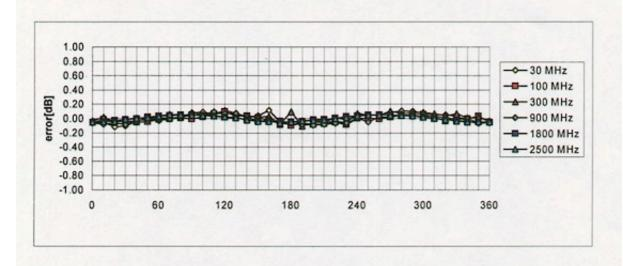
Axial Isotropy Error < ± 0.2 dB
