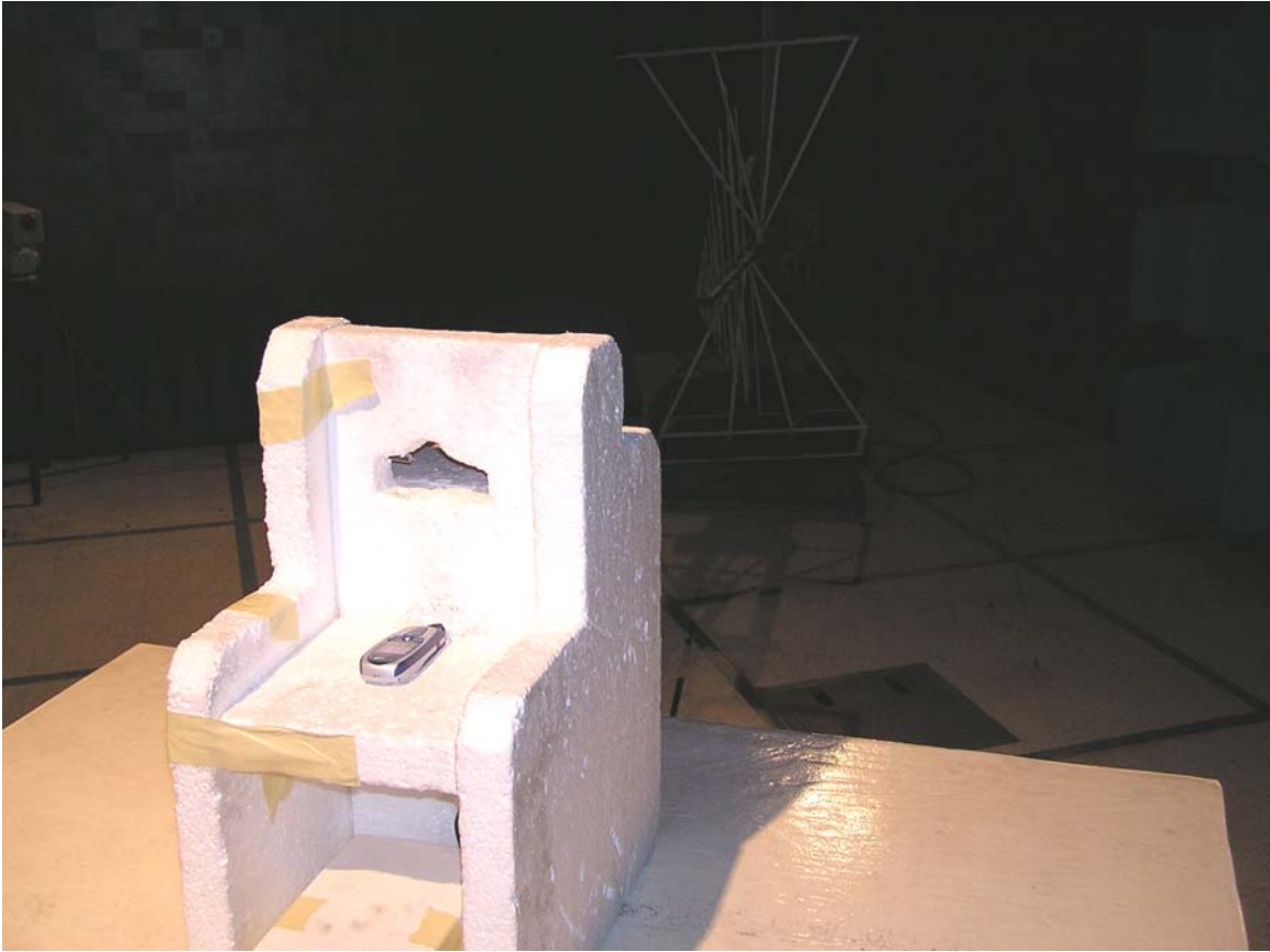
Test setup – Radiated Emissions
