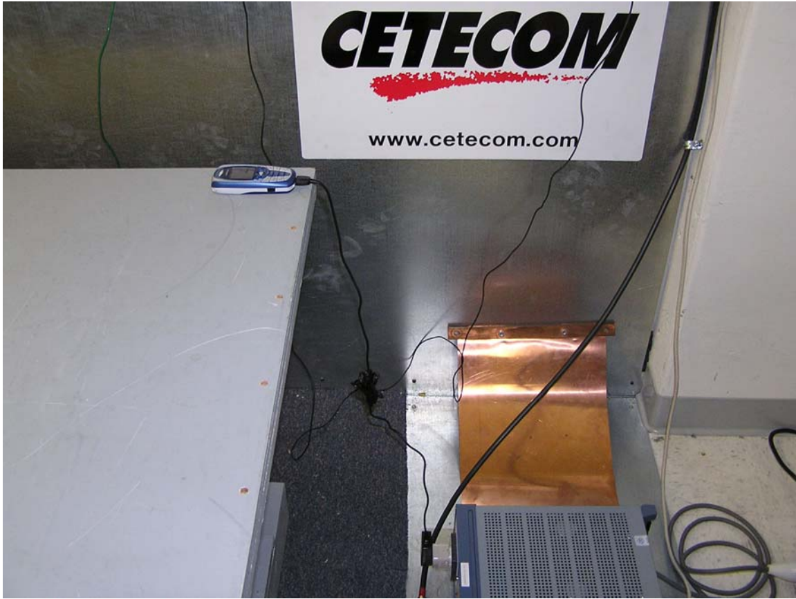
Test setup – AC Line Conducted Emissions
