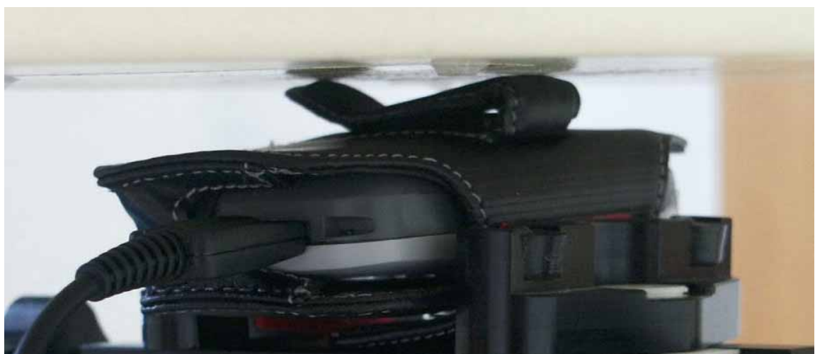
Fig. 27: Body worn configuration, GPRS Class 8 with data cable and FCL600, antenna towards the phantom (13 mm distance).
