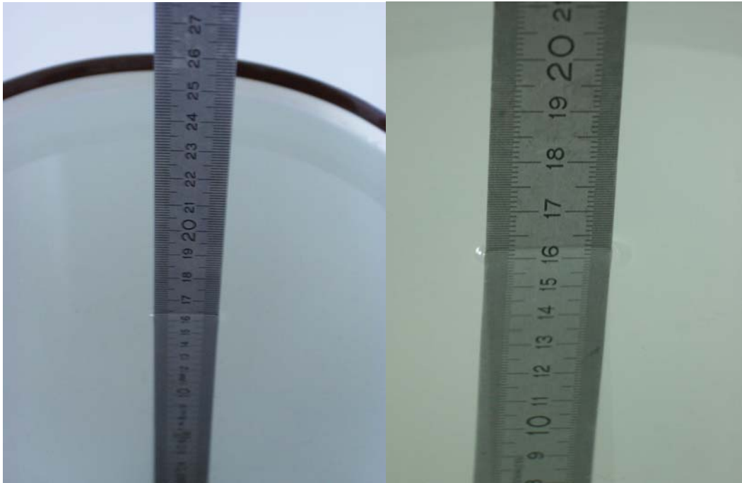
Fig. 26: Liquid depth for PCS 1900 Head and Body measurements.
