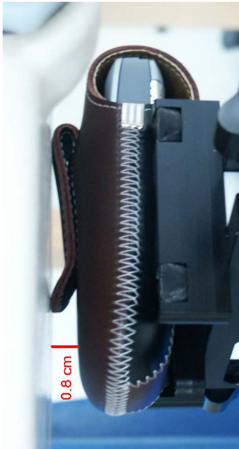
Fig. 25: Body worn configuration, GPRS mode (2 TX slots) with beltcase.
