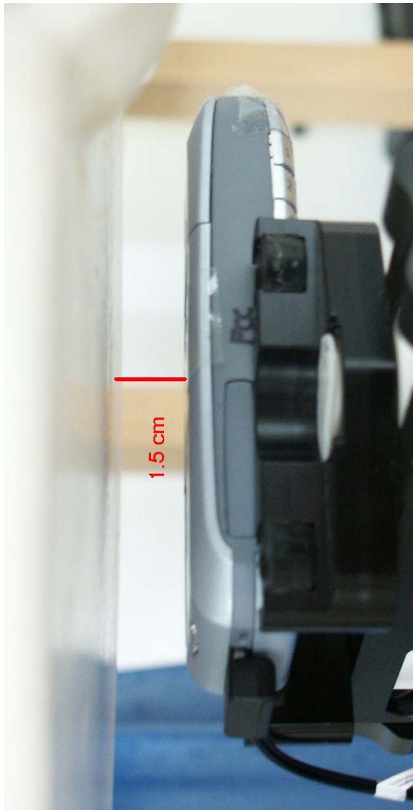
Fig. 23: Body worn configuration, GSM mode (1 TX slot).
