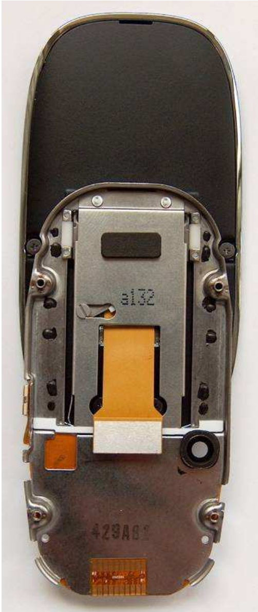
Disassemble Step 4: Slider Upper Case Back, Open
