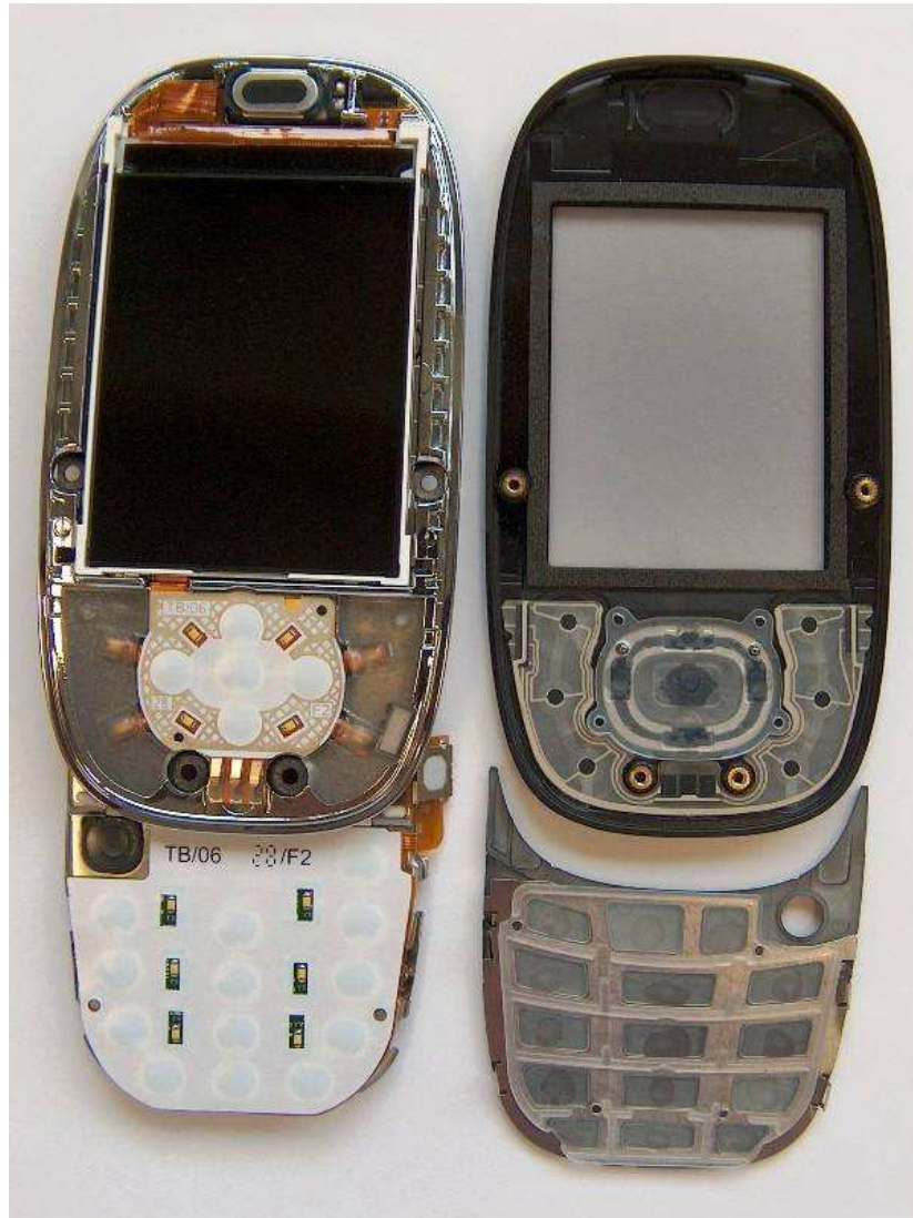
Disassemble Step 2: Front Cover and Keypad separated from Slider
