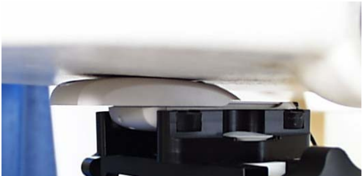
Fig. 48: Body worn configuration, slider up with headset, display towards the phantom.
