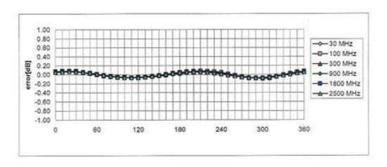
Axial Isotropy Error < ± 0.2 dB
