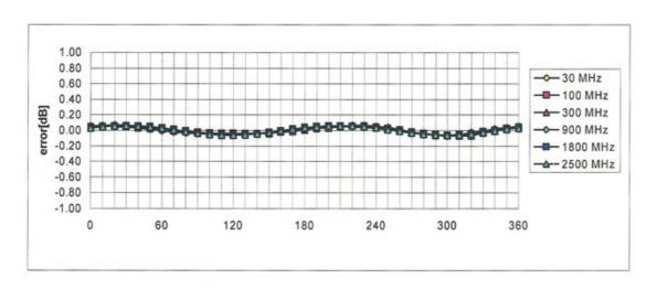
Axial Isotropy Error < ± 0.2 dB
