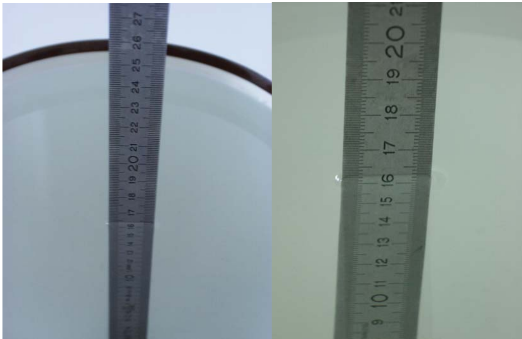
Fig. 35: Liquid depth for PCS 1900 Head and Body measurements.
