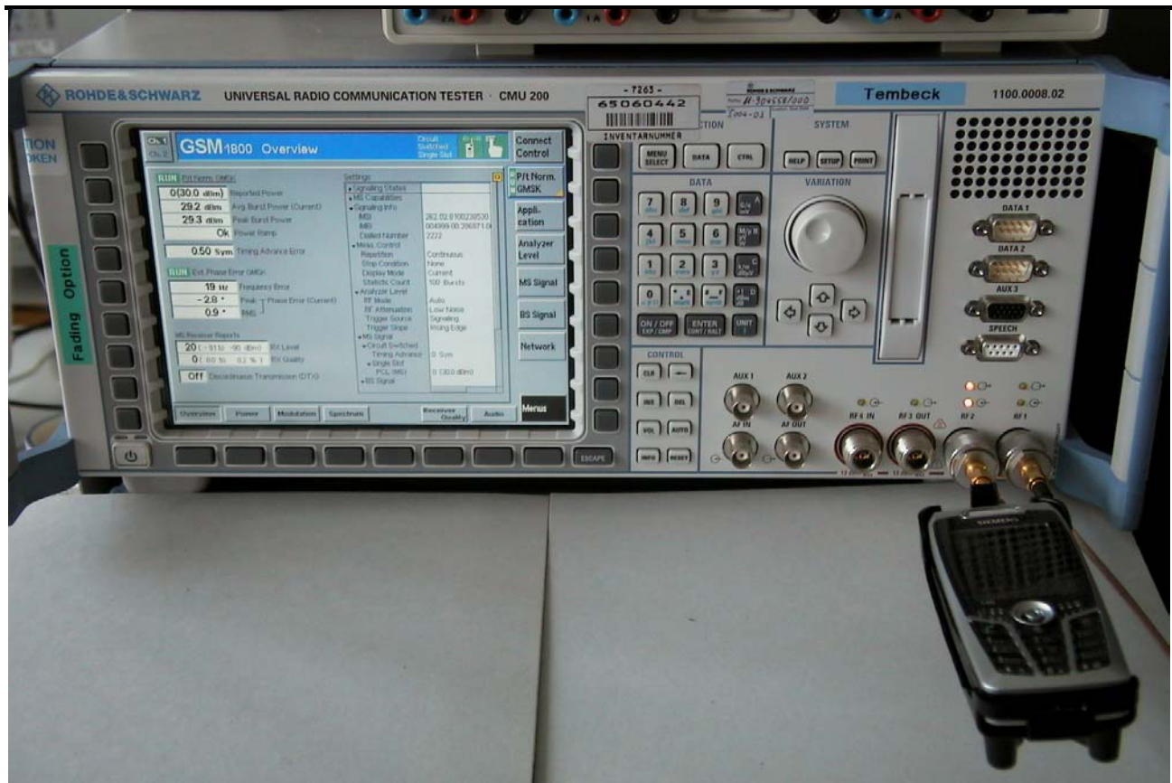
Figure 2: Set-up for conducted power measurement
