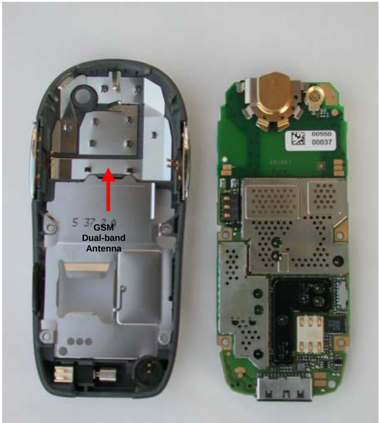
S56 Disassembly step 2: GSM Dual-band Antenna
