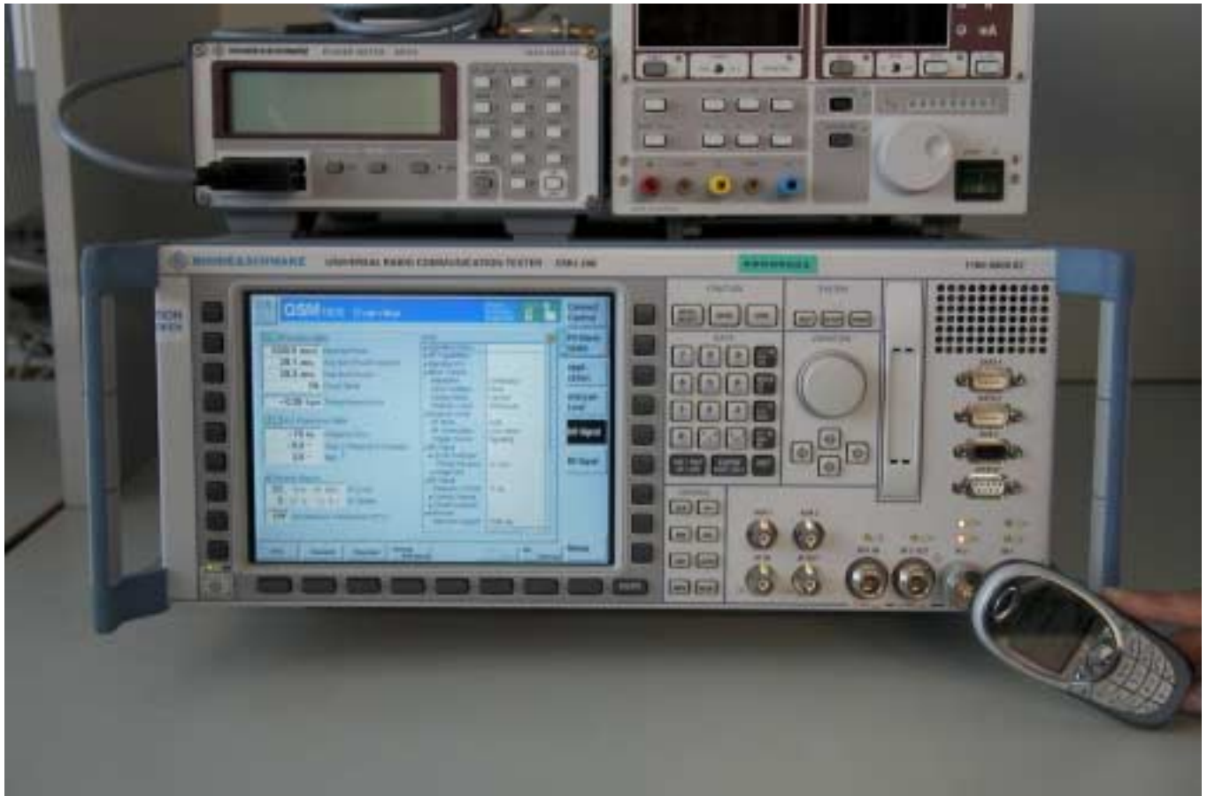
Fig. 2: Set up for conducted power measurement.
