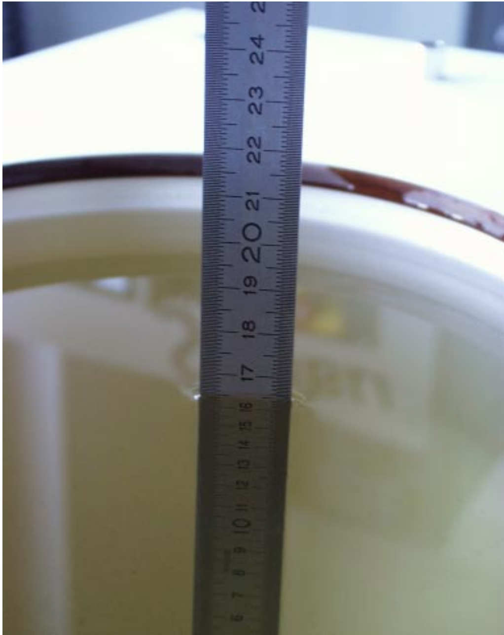
Current liquid depth (16.5 cm) for the 800MHz/900MHz head liquid
