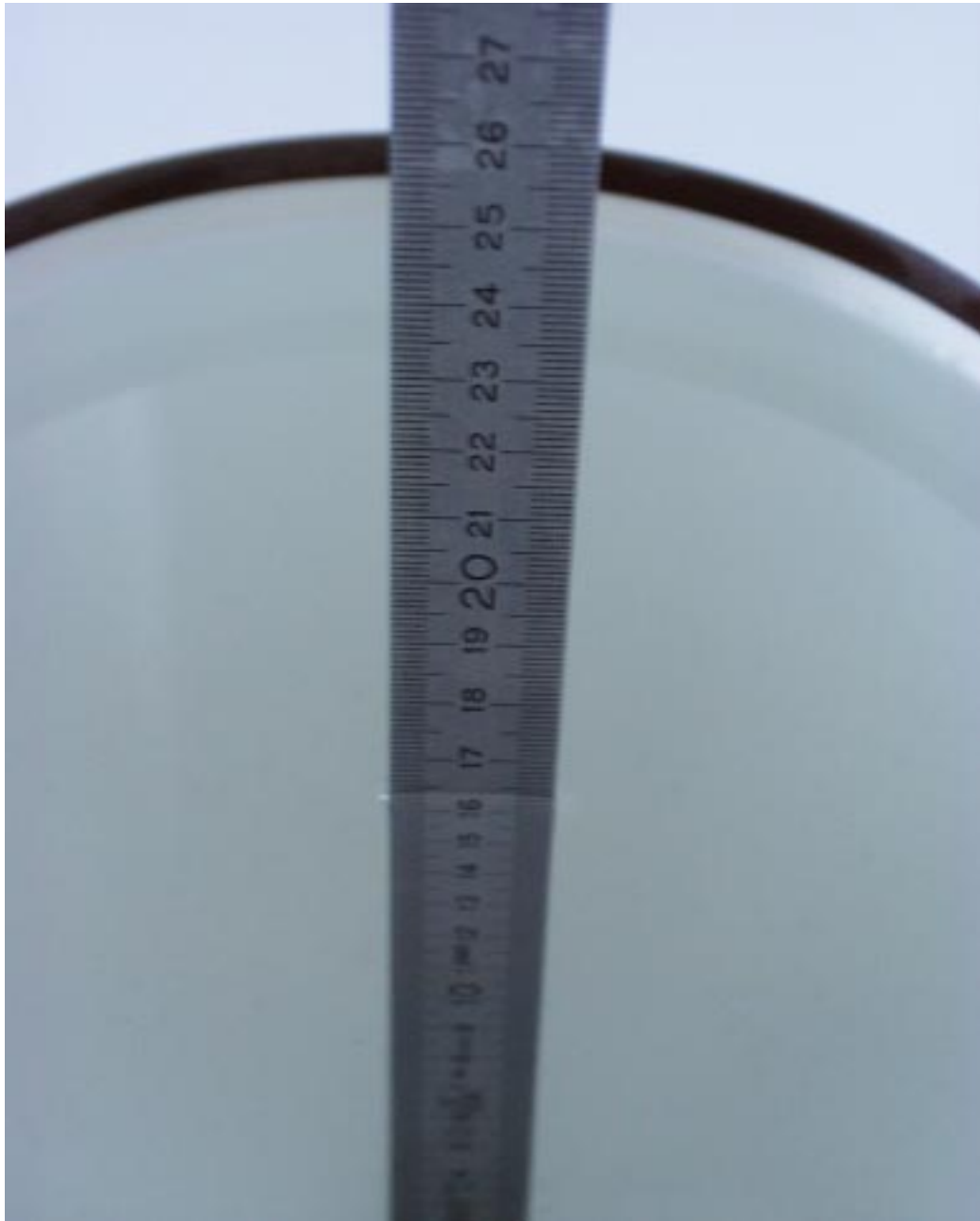
Current liquid depth (16.4 cm) for the 1800MHz/1900MHz head liquid
