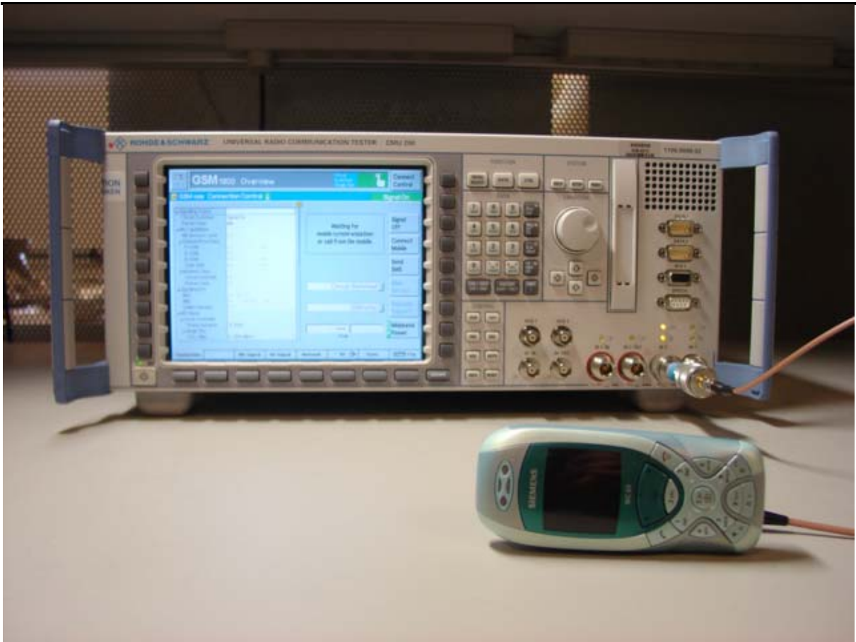
Figure 2: Set-up for conducted power measurement
